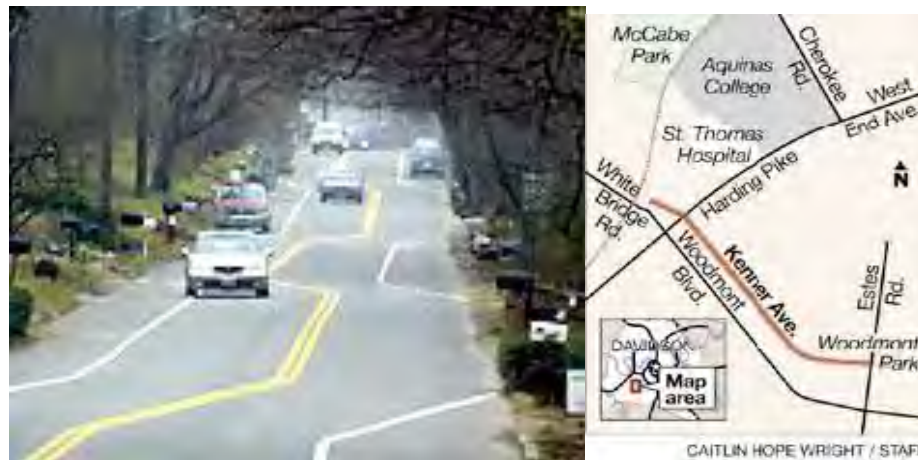
Figure 4: Use of pavement marking to create chicane (Hamburg, 2005)
