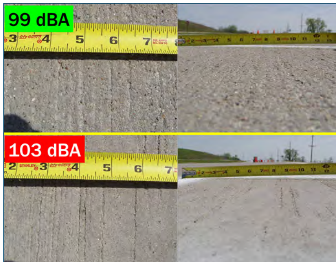
Figure 10. Variability of drag texture surface and its effect on overall OBSI level
