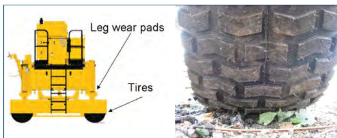
Figure 52. Side view of texture-cure machine on tires, and close up of tire
