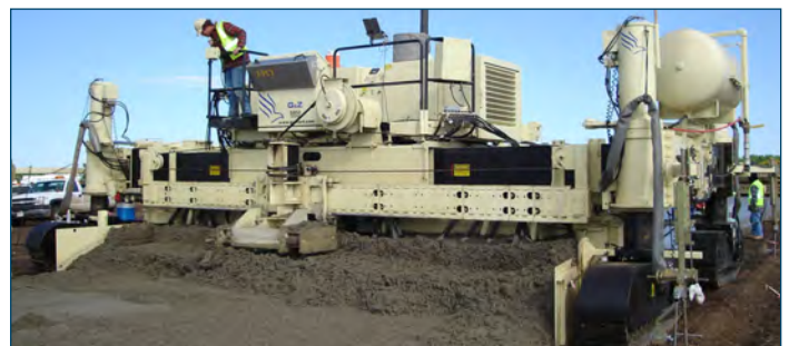
Figure 40. Spreader (plow) at the front of a paver
