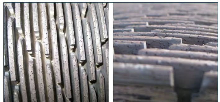
Figure 30. Diamond grinding head showing blades (with embedded diamonds) separated by spacers
