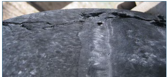
Figure 62. Cracked drive wheel
