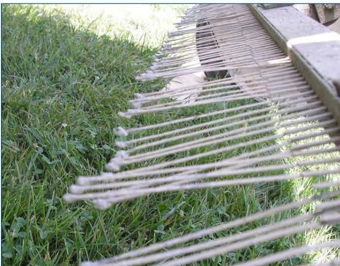
Figure 21. Bent tines on rake that can lead to nonuniform tine depth
