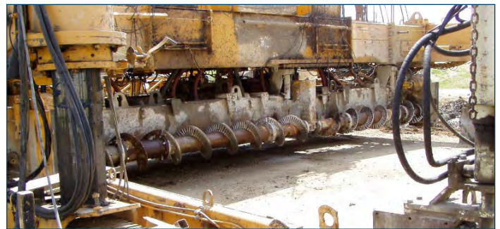
Figure 39. Auger located at the front of a paver
