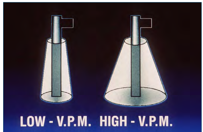
Figure 42. A difference in vibrator frequency will influence the volume of concrete that is consolidated
