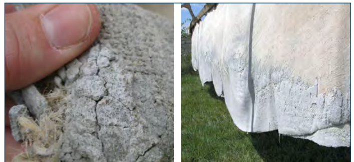
Figure 29. Hardened mortar on drag materials
