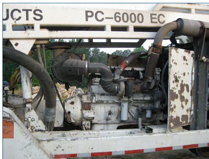
Figure 64. 500 HP, 15 liter engine used to power grinding head
