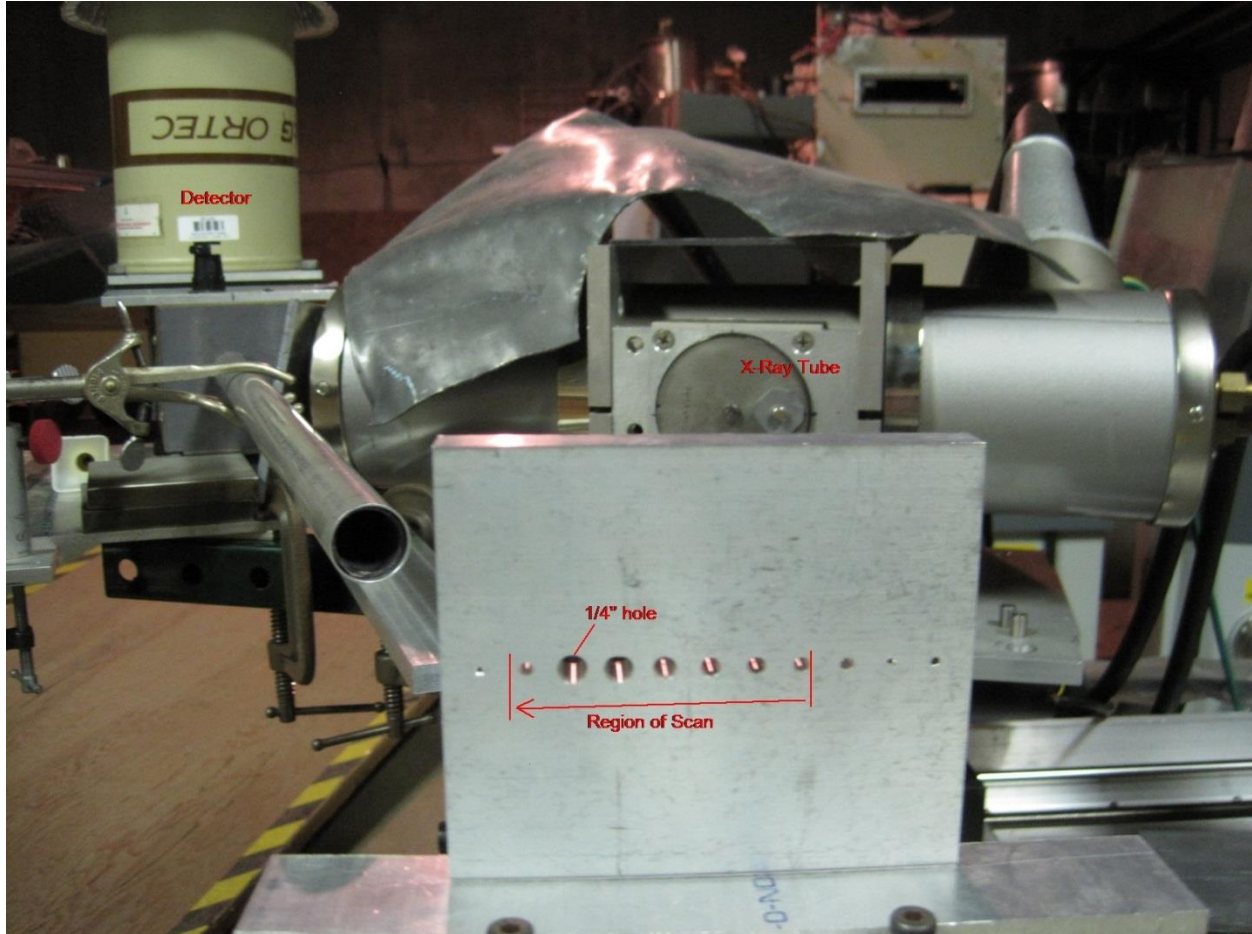
Figure 6. Setup used for x-ray backscatter studies
