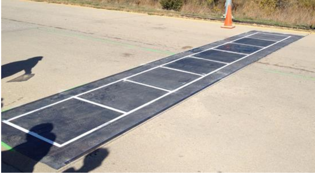
Figure 1. Rubber mat used to capture salt by grid sample
