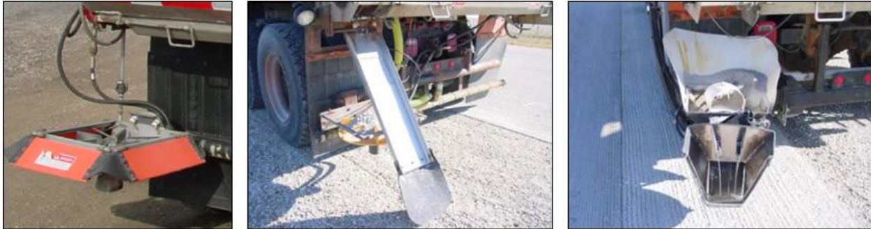
Figure 2. Salt spreaders evaluated (standard on the left, chute in the middle, and zero-velocity on the right)
