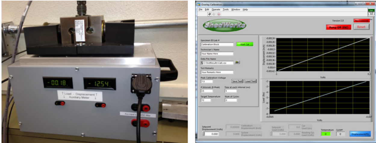
Figure 3-5. The New OT Calibration Kit and Examples of Linear Graphical Screen Plots.
