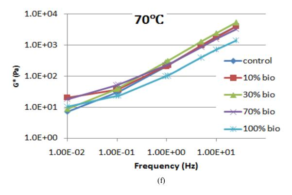
Figure 5-12: Complex shear modulus (|G\*|) of different asphalt binders at temperatures from 40°C to 70°C
