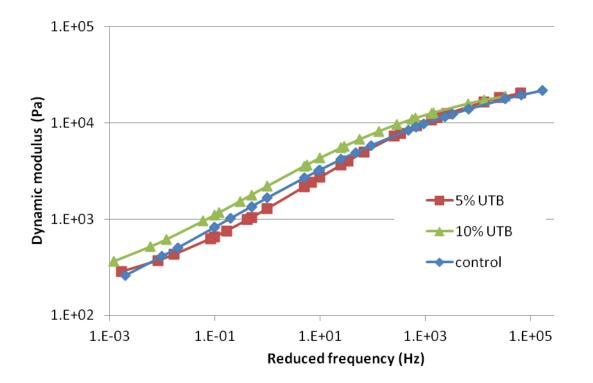
Figure 6-2: Dynamic modulus master curve plot for control asphalt mixture, 5% and 10% UTB modified asphalt mixture
