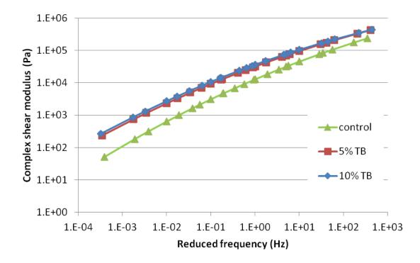
Figure 4-17: G\* master curve plot for control binder and 5% and 10% TB modified asphalt binders after PAV aging
