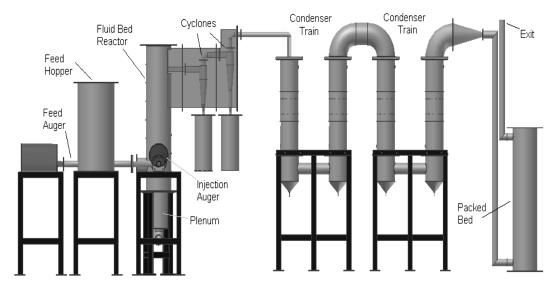
Figure 2-1: A schematic of the fluidized bed fast pyrolysis unit used in this research
