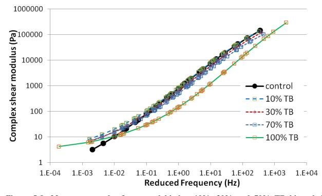
Figure 5-9: Master curve plot for control binder, 10%, 30% and 70% TB bioasphalt binders in the temperature range of 40°C to 70°C.
