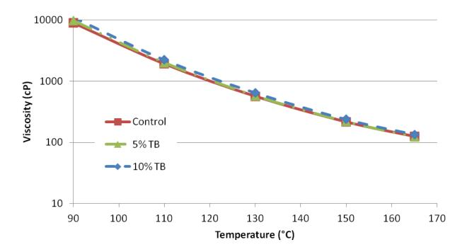
Figure 4-5: RV test results of control binder, 5%, and 10% UTB modified binders, after RTFO aging
