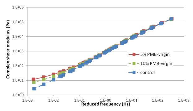
Figure 4-10: G\* master curve for control binder, 5% and 10% PMB modified asphalt binders before RTFO aging
