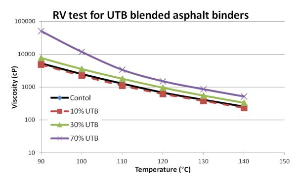
Figure 5-4: RV results for control asphalt binder PG 58-28, and 10%, 30%, 70% and 100% UTB bioasphalt binders after RTFO aging
