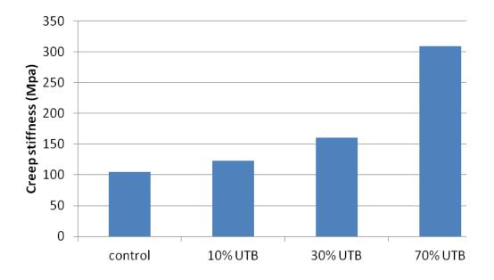
Figure 5-16: Creep stiffness of control binder, 10%, 30% and 70% UTB bioasphalt at 60s during BBR test
