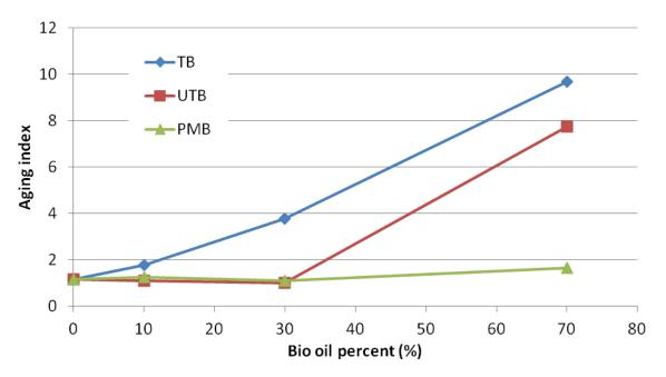
Figure 5-15: Aging indexes of control binder, 10%, 30% and 70% bioasphalt binders after RTFO aging in temperature range of 40°C to 70°C
