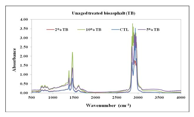
Figure 3-4: FTIR spectra for control and treated bio oil modified PG 58-28 asphalt binder at unaged condition
