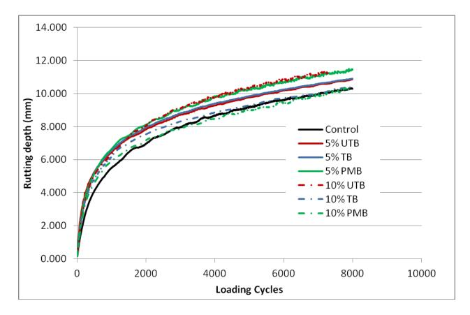
Figure 6-6: The APA test results for control HMA mixture and bio oil modified HMA mixture at 58°C
