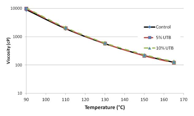
Figure 4-4: RV test results of control binder, 5%, and 10% UTB modified binders, after RTFO aging
