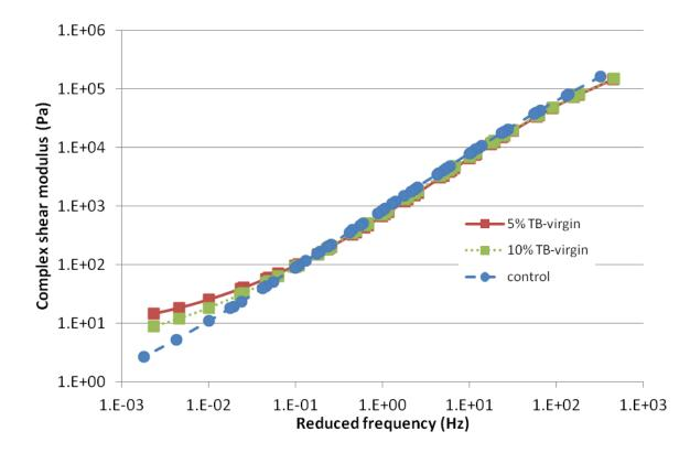
Figure 4-9: G\* master curve for control binder, 5% and 10% TB modified asphalt binders before RTFO aging
