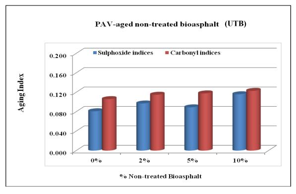
Figure 3-9: Bar chart of aging indices for PAV-aged control and untreated bioasphalt
