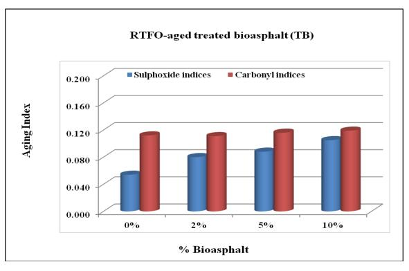
Figure 3-8: Bar chart of aging indices for RTFO-aged control and treated bioasphalt
