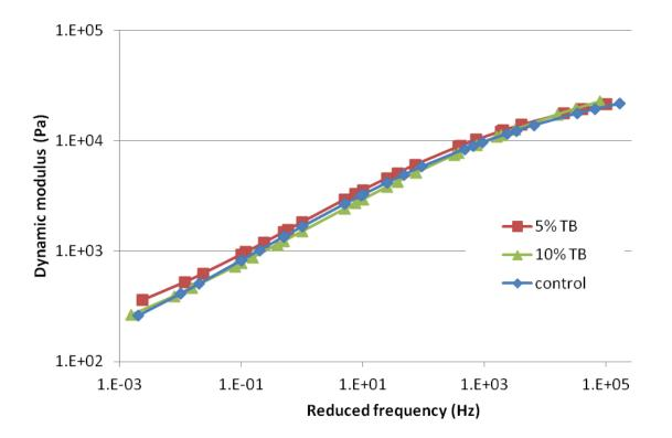
Figure 6-3: Dynamic modulus master curve plot for control asphalt mixture, 5% and 10% TB modified asphalt mixture
