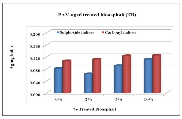
Figure 3-10: Bar chart of aging indices for PAV-aged control and treated bioasphalt
