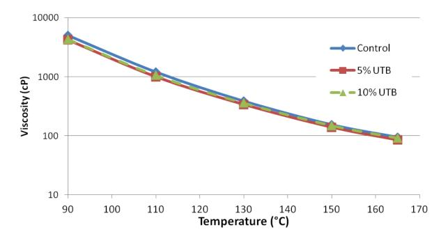
Figure 4-1: RV test results for control binder, 5%, 10% and 100% UTB modified asphalt binders before RTFO aging
