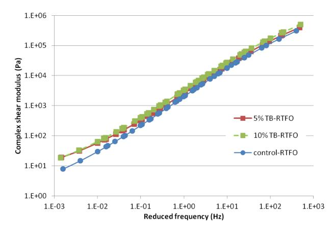
Figure 4-12: G\* master curve plot for control binder, 5% and 10% TB modified asphalt binders after RTFO aging
