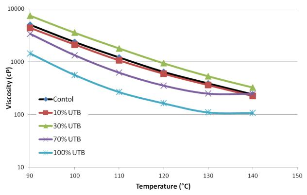
Figure 5-1: RV test results for control binder, 10%, 30%, 70% and 100% UTB bioasphalt binders
