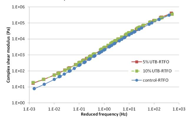
Figure 4-11: G\* master curve plot for control binder, 5% and 10% UTB modified asphalt binders after RTFO aging
