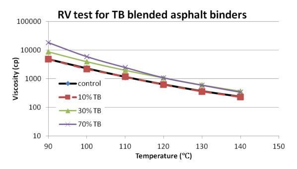
Figure 5-5:RV results for control asphalt binder PG 58-28, and 10%, 30%, 70% and 100% TB bioasphalt binders
