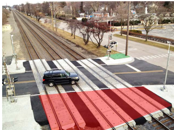
Figure 14. Non-Traffic Area Established for Snowfall False Detection Tests
