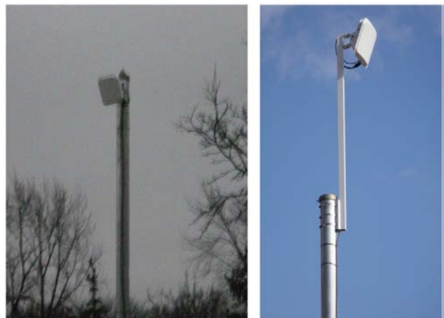
Figure 12. Radar Mounted at 14.5 Ft versus 19.5 Ft
