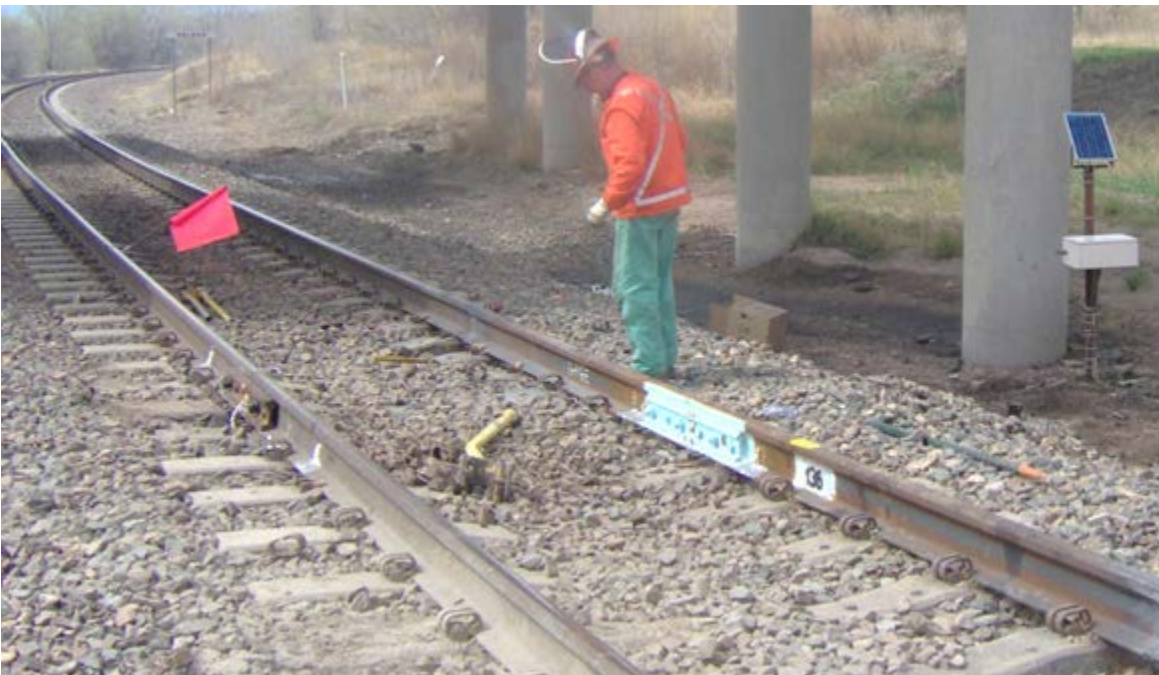
Figure 9. Thermal Stress – Temperature Data Collection on a Western Railroad, Colorado Springs, CO
