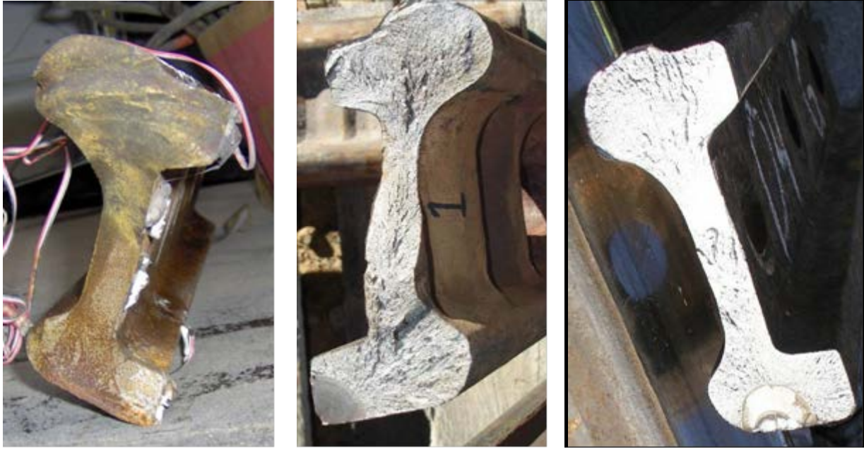
Figure 28. (left) Yield Failure (brittle failure), (middle) Fatigue Crack, (right) Crack Started at Fault
