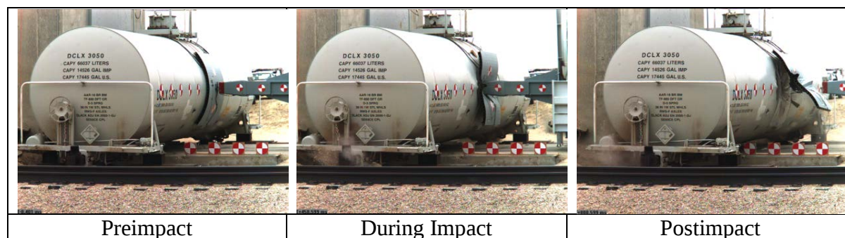
Figure 37. Series of Images Showing Side Impact Progression
