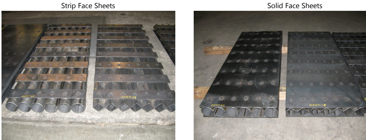
Figure 12. Photos of Panels for Three-Point Bend Testing
