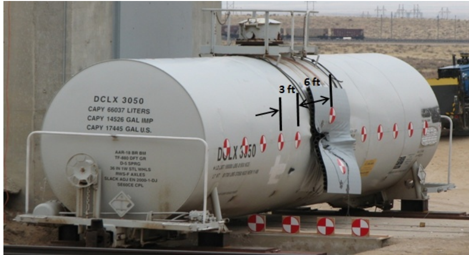
Figure 38. Tank Car and Panel after Impact
