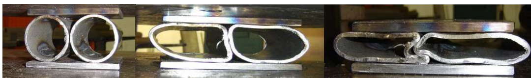
Figure 7. Photos of Round-Tube Panel during Crushing
