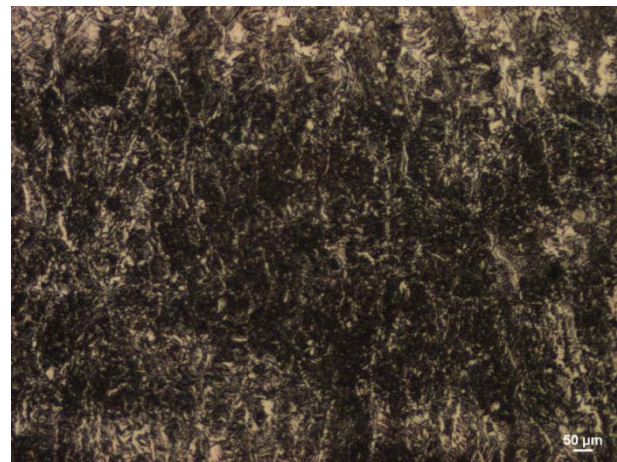
Figure 59. HAZ in TC128-B Steel
