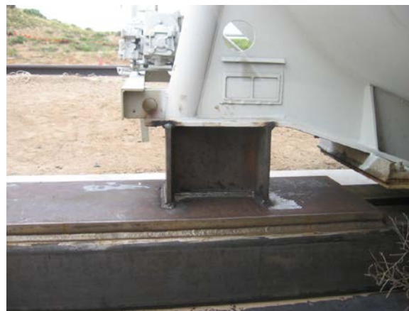
Figure 27. Welded Beam Connecting the Tank Car to the Skid System
