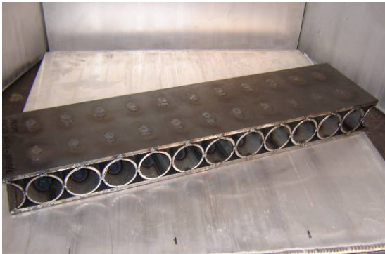
6"x2'x2" Round Tube Core Test Article (P3)
