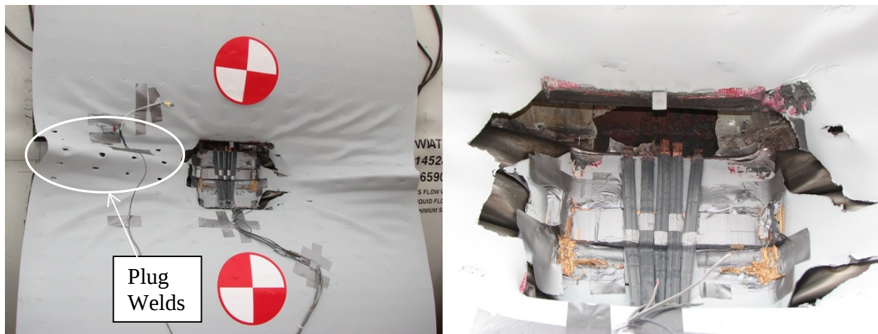
Figure 39. Damage on Protective Panel – Impact Side
