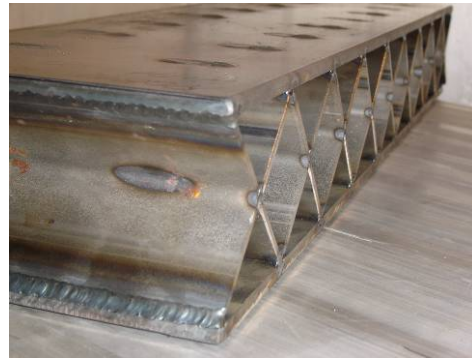
Figure 10. Photos of Manufactured Panels for Uniaxial Compression Tests
