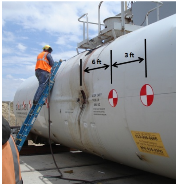
Figure 42. Dent in the Jacket
