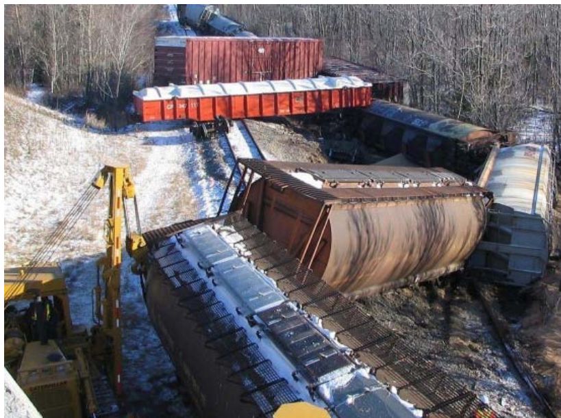
Figure 2.10. Derailed railcar lateral displacement due to embankment
