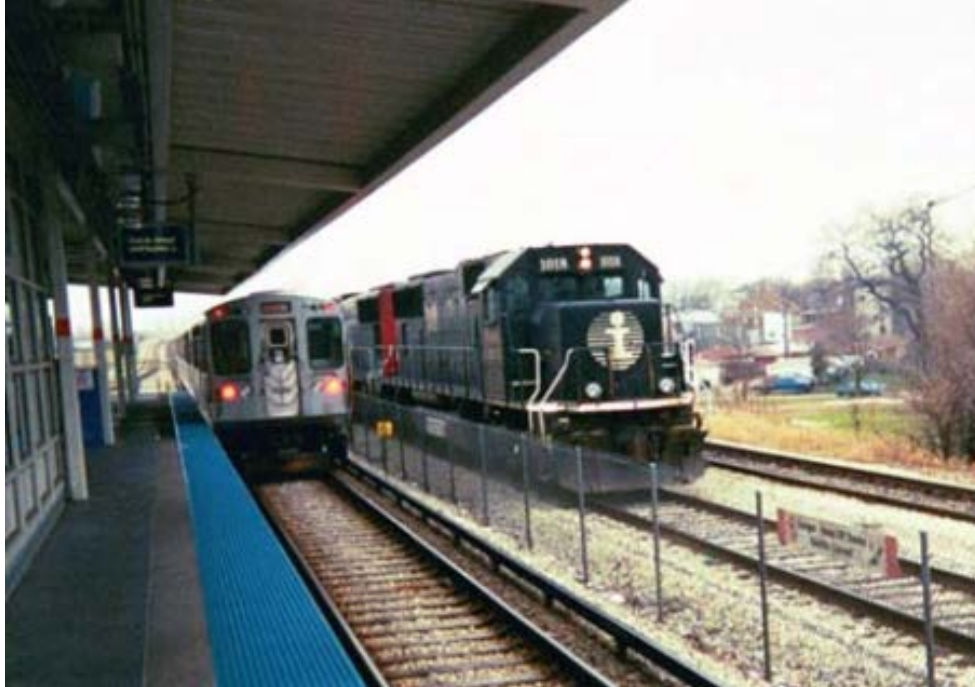
Figure 2.3. CTA and CN trains sharing a corridor with 13-foot track center distance
