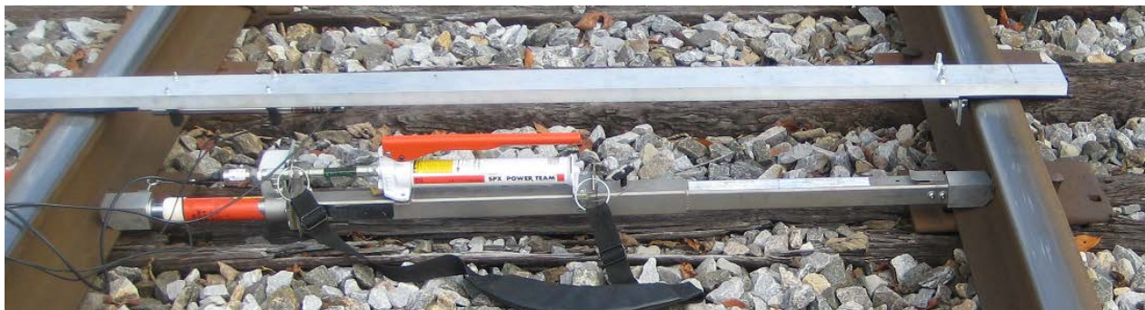
Figure 1. The Portable Track Loading Fixture (PTLF) in Use for Testing
