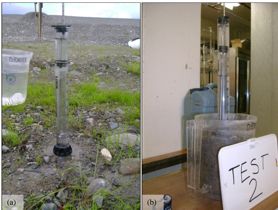
Figure 11. Tension infiltrometer tests (a) in the field and (b) in the laboratory.
