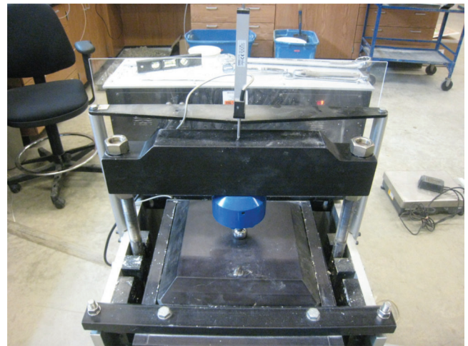
Figure 3.4 Load cell and LVDT positioned properly after the top plate cap is placed over the aggregate layer.
