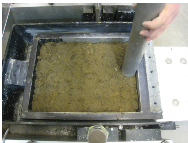
Figure 3.1 Soil placed in the lower shear box and compacted in three layers.
