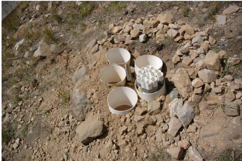
Figure 17. Overview of fertility release incubation columns during construction. Tubes left in the field were placed with tops level to the ground surface.
