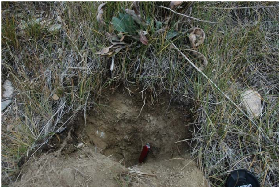
Figure 30. An example soil pit on a lower revegetation cover plot showing extensive root development into the previously non-living decomposed granite substrate.
