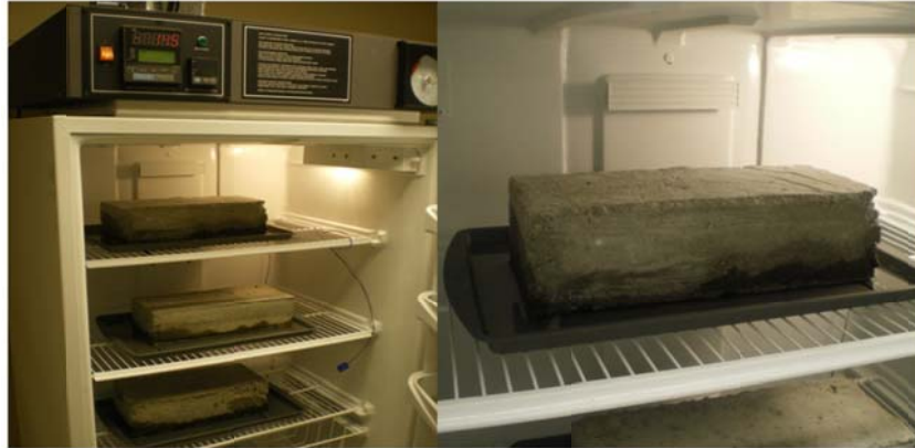
Figure 6.7. FRP reinforced concrete specimens undergoing free-thaw exposure
