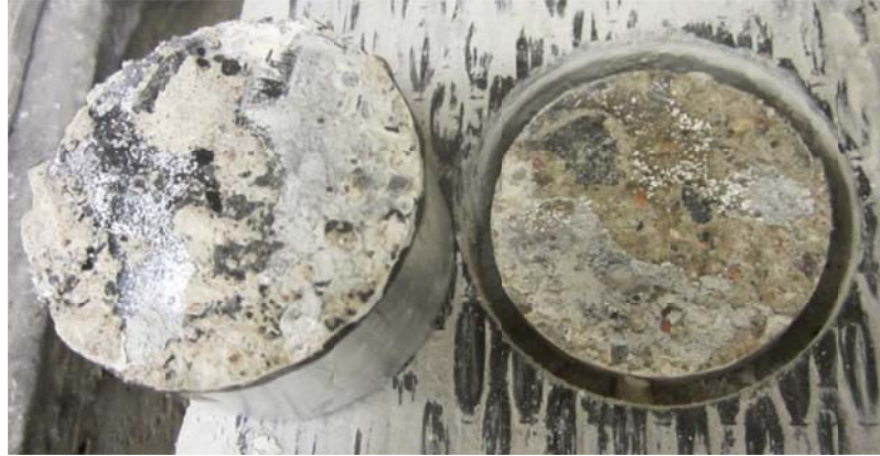
Figure 6.32. Presence of moisture on dollies
