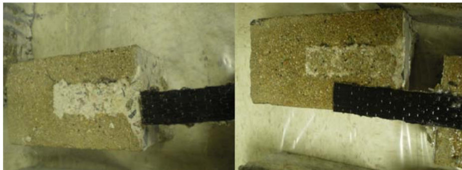
Figure 6.29. Beam #1 (left) vs. beam #8 (right) failure
