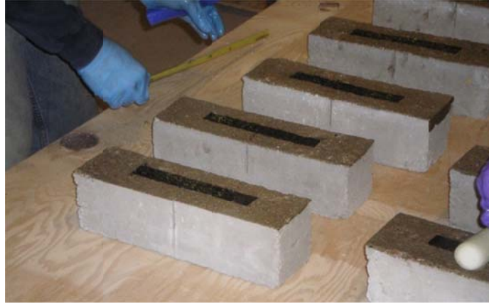
Figure 6.15. Concrete beams reinforced with CFRP
