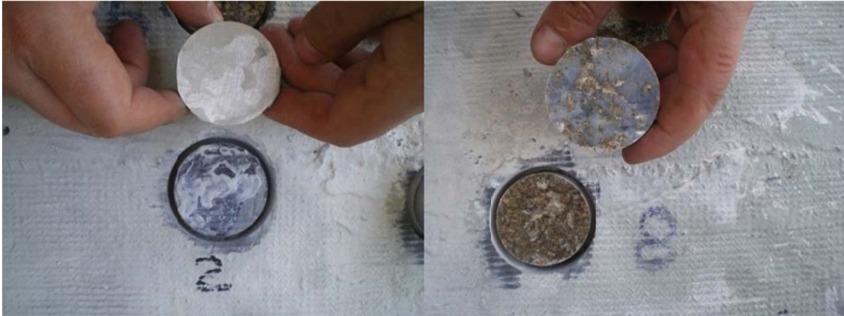
Figure 3.14. Failure Mode A: bonding adhesive failure at loading fixture (on left), failure Mode E: adhesive failure at CFRP/substrate adhesive interface (on right)
