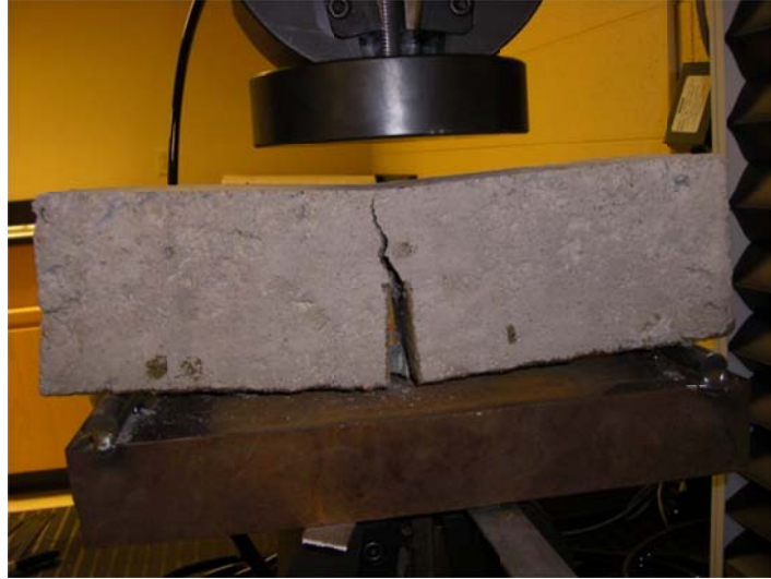
Figure 6.22. Beam following crack failure
