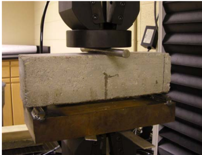
Figure 6.16. Beam fixture and specimen
