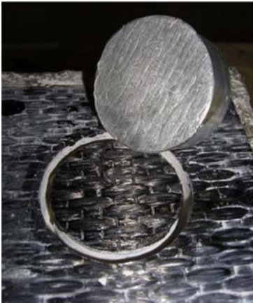
Figure 6.18. Pull-off Mode A failure
