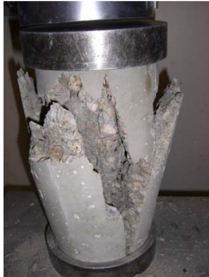
Figure 6.17. Characteristic failure for compression tests
