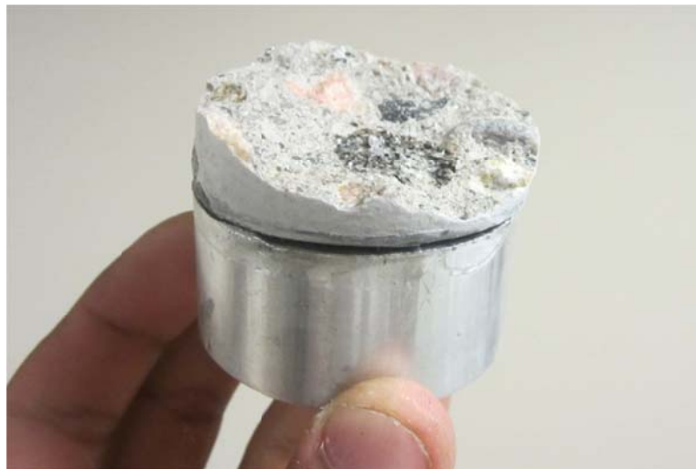
Figure 6.31. Mode G failure in dolly #20
