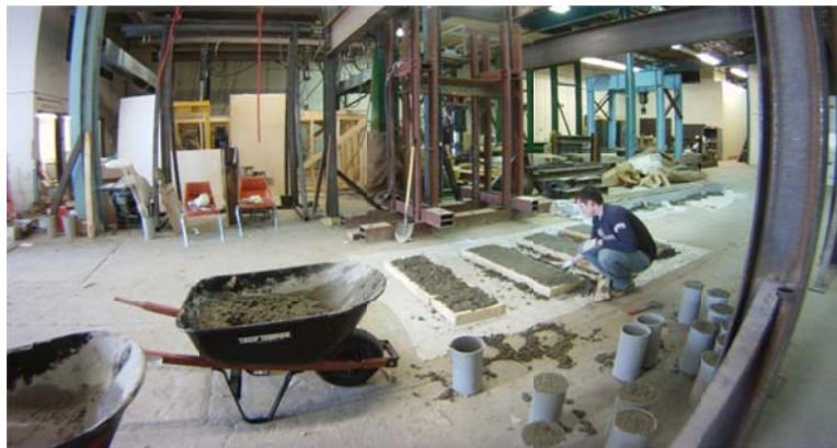
Figure 6.8. Casting of concrete specimens
