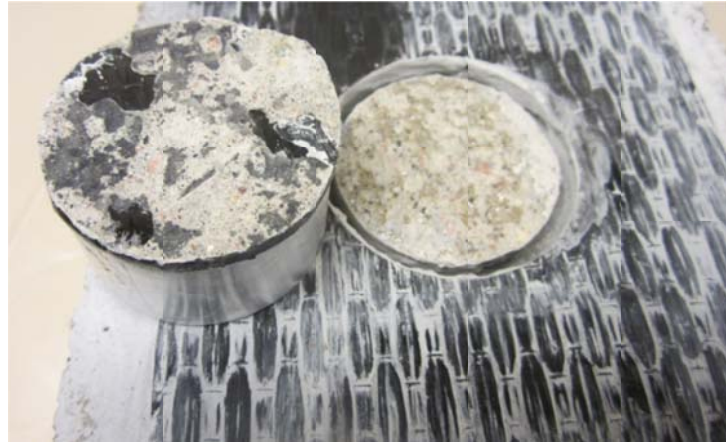
Figure 6.30. Representative Mode F failure for Stage 2
