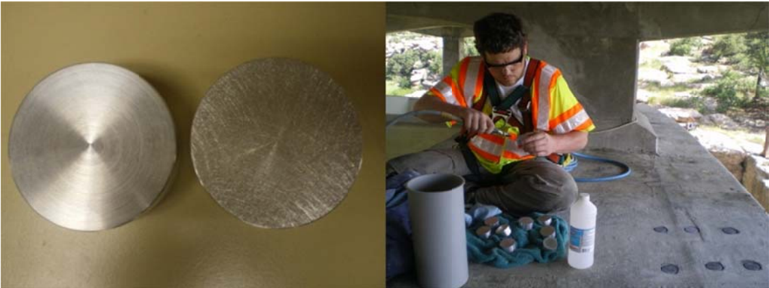
Figure 3.10. Aluminum pucks before and after sanding with 40 grit sandpaper and preparing the aluminum pucks way up high on the arch
