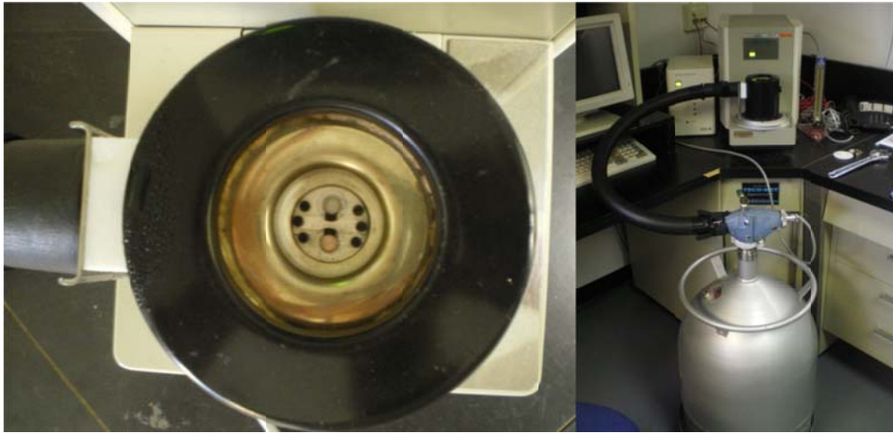
Figure 4.12. DSC specimen chamber and DSC with liquid nitrogen
