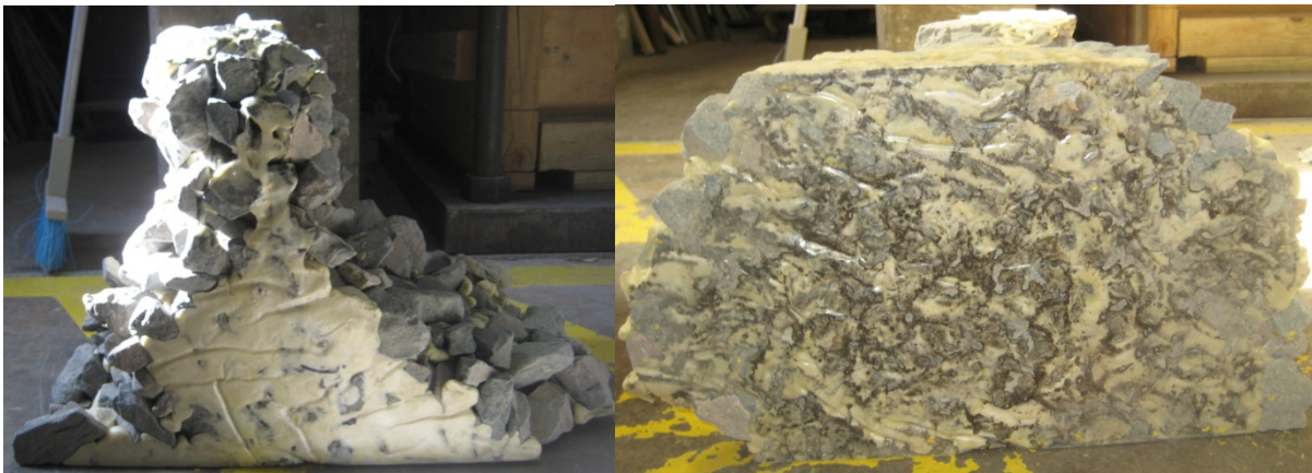
Appendix Figure 27: PSB from percolation injection into ballast layer prototype.
