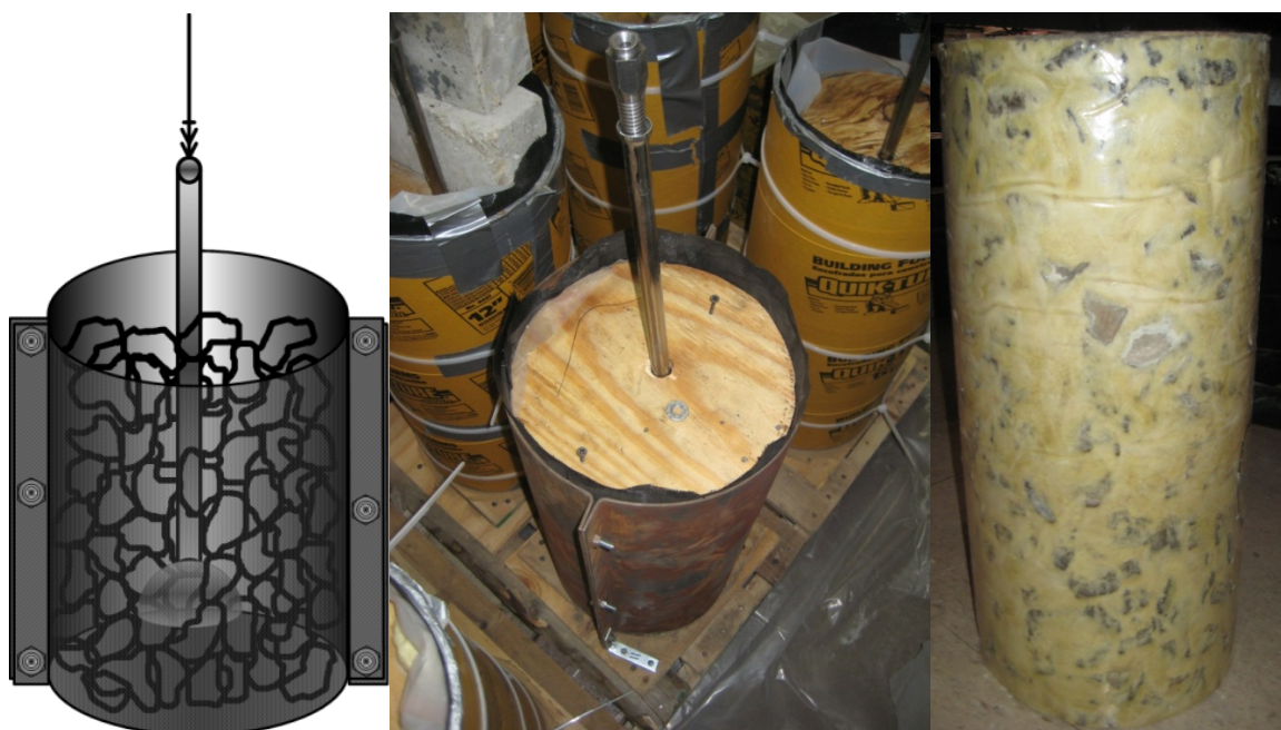
Figure 3.3.2: Diagram of injection mold (left), picture of specimen fabrication molds (middle), picture of PSB cylindrical specimen (right).
