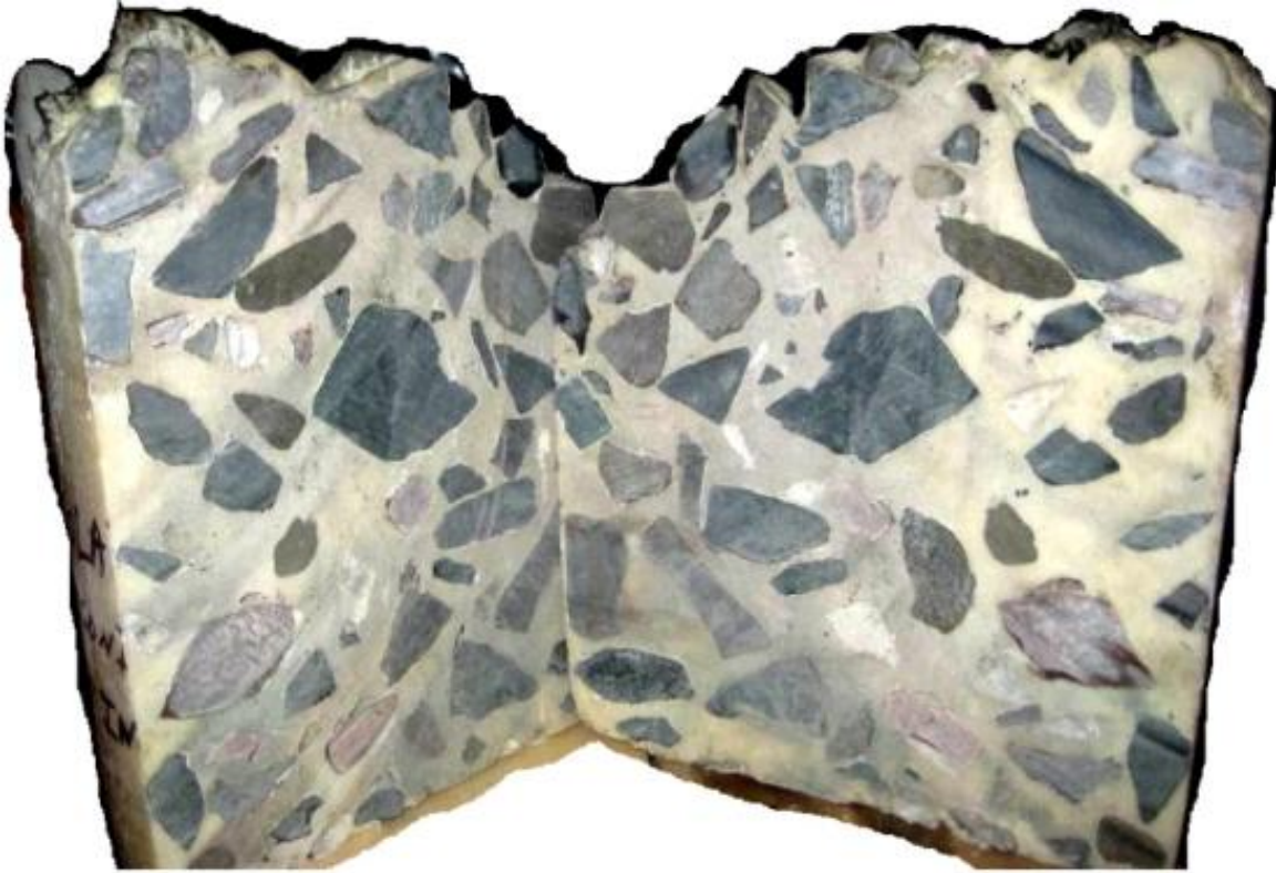
Figure 3.2.4: A PSB specimen cut in half shows complete void filling by the expanding foam and coherence of the two materials after concrete masonry saw was used for cutting.
