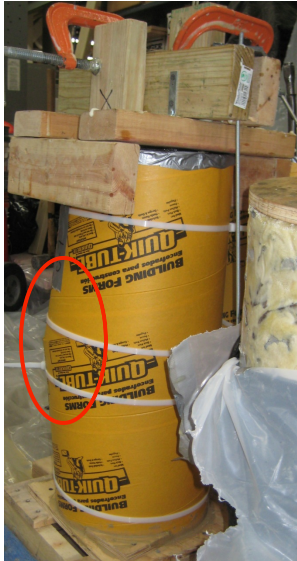
Appendix Figure 25: Fabrication error in PSB Cylinder # 6, considered outlier in analysis.
