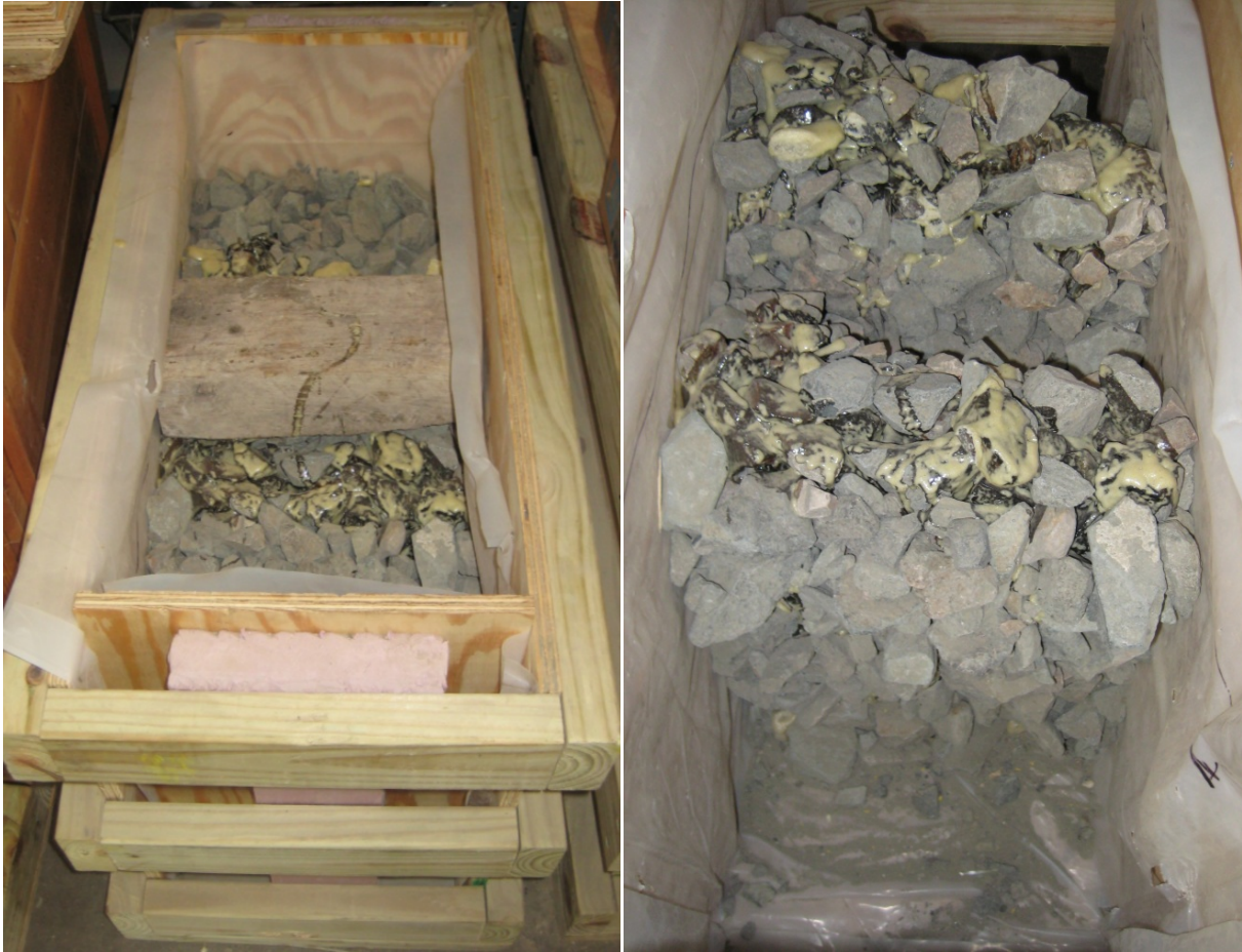
Appendix Figure 11: Picture of ballast layer prototype with RPF percolation-injection along the surface (left) and resulting stabilized areas after removing loose ballast (right).
