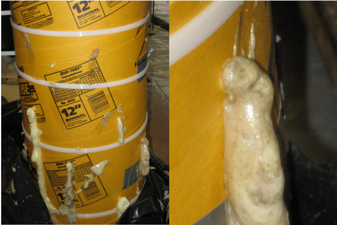
Appendix Figure 26: Pictures of fabrication of PSB fouled ballast specimen. Pressure relief holes were drilled into fabrication mold where small amounts of soil mixed with RFB expelled from the specimen during RPF expansion/reaction.
