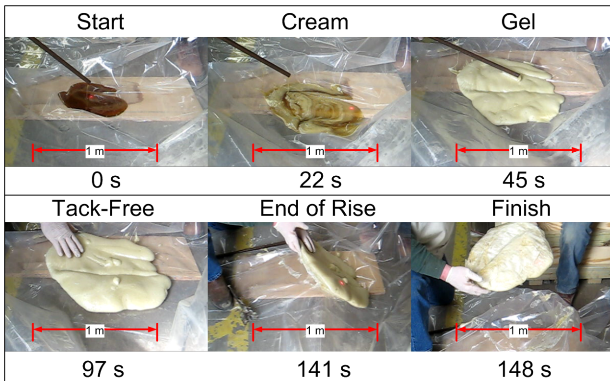
Appendix Figure 4: Pictures displaying each phase of the RPF reaction process with timings displayed for a 35°C starting temperature.
