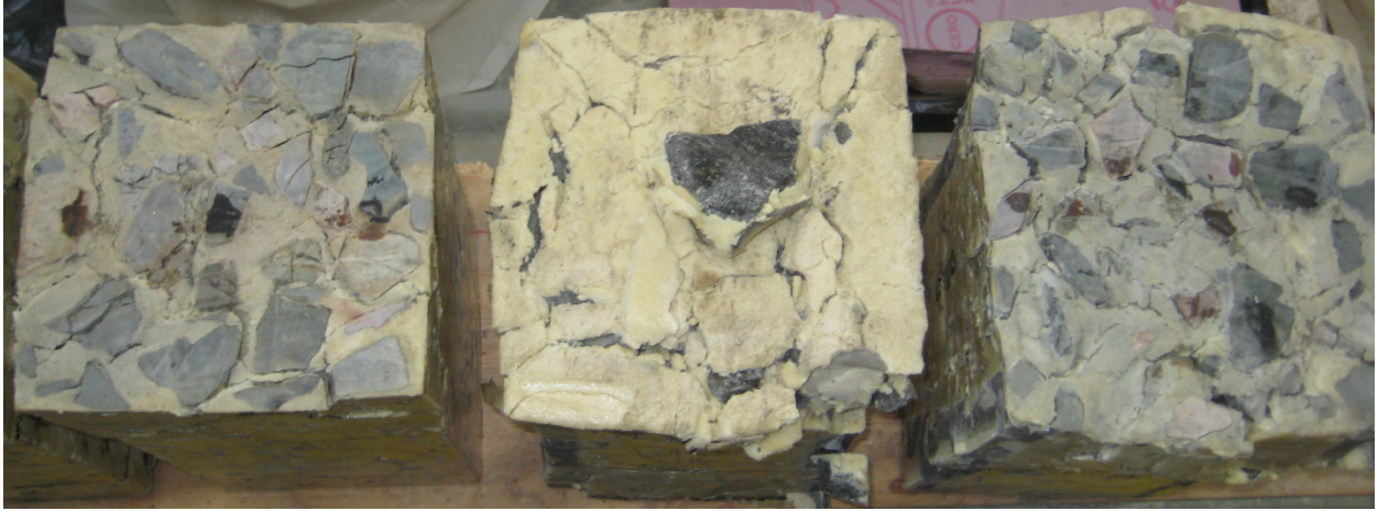
Appendix Figure 29: PSB prism specimens after failure in unconfined compression testing.
