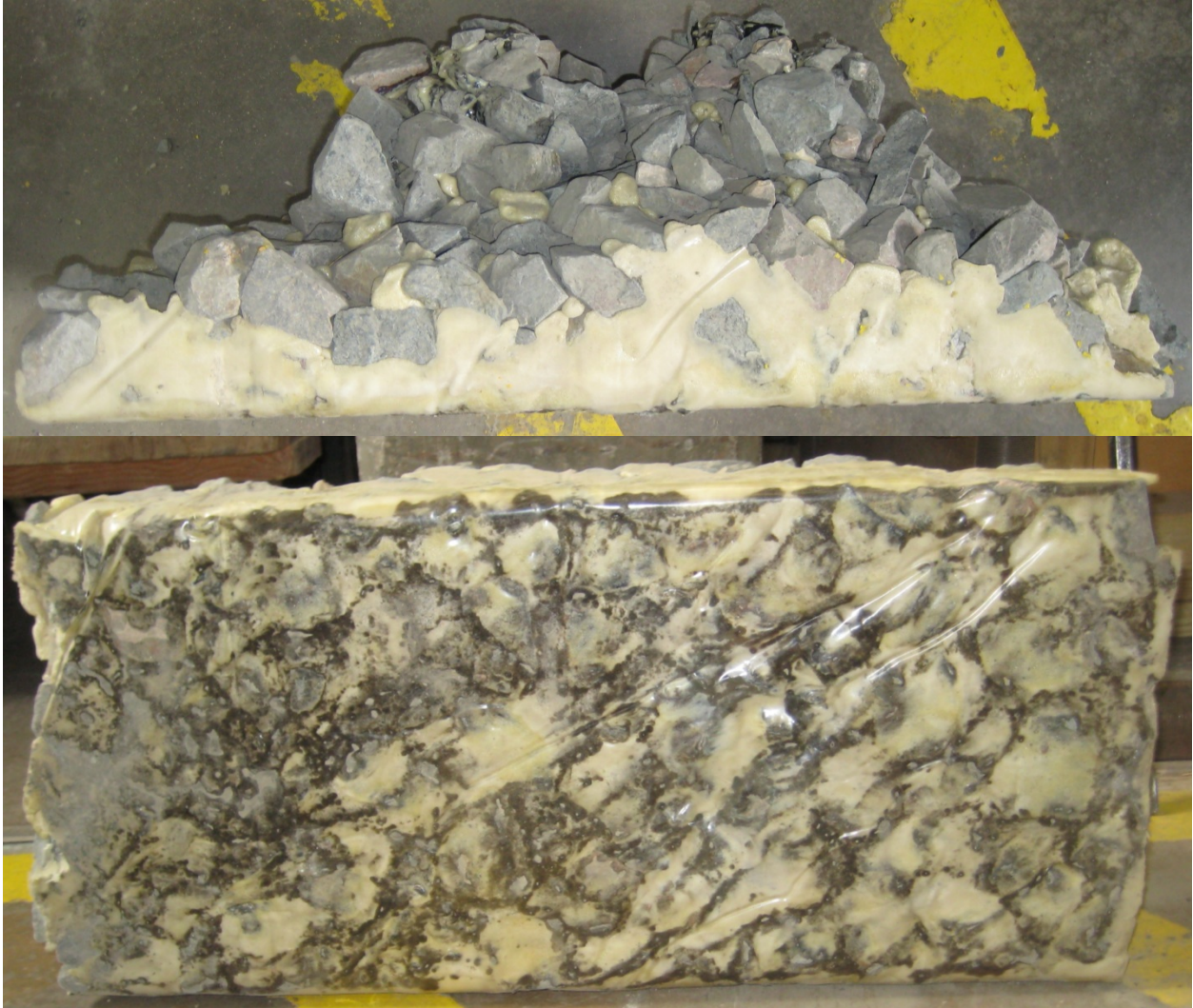
Appendix Figure 12: Photo of side-view of prototype with RPF subsurface-injection into ballast layer prototype (top) and base of injected ballast layer prototype (bottom). Effective height (top) = 20 cm and base dimensions (bottom) = 0.3 m x 0.66 m.
