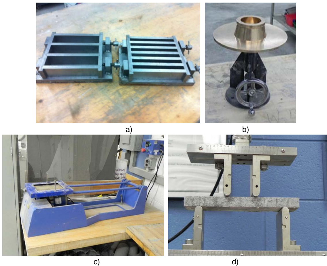
Figure 14. The Equipment Setup Used in ECC/SECC Study: a) Six-Gang Mold used for ECC Specimens; b) Flow Table; c) Jolting Table; d) The Setup of 4-Point Bending Test
