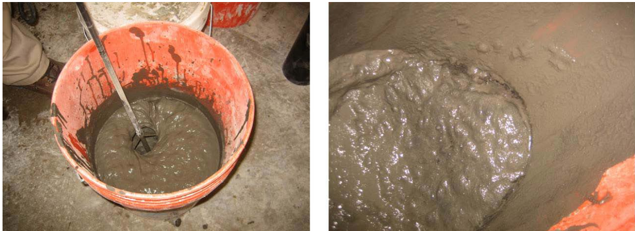
Figure A1. Typical Consistency of an ECC (Shown is Mix 4)
