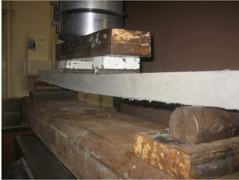
Figure A3. Flexural Test Setup of Preliminary Trial Mixes
