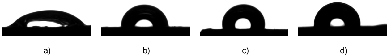
Figure 21. The Contact Angle of Mortar with a Single Coat
