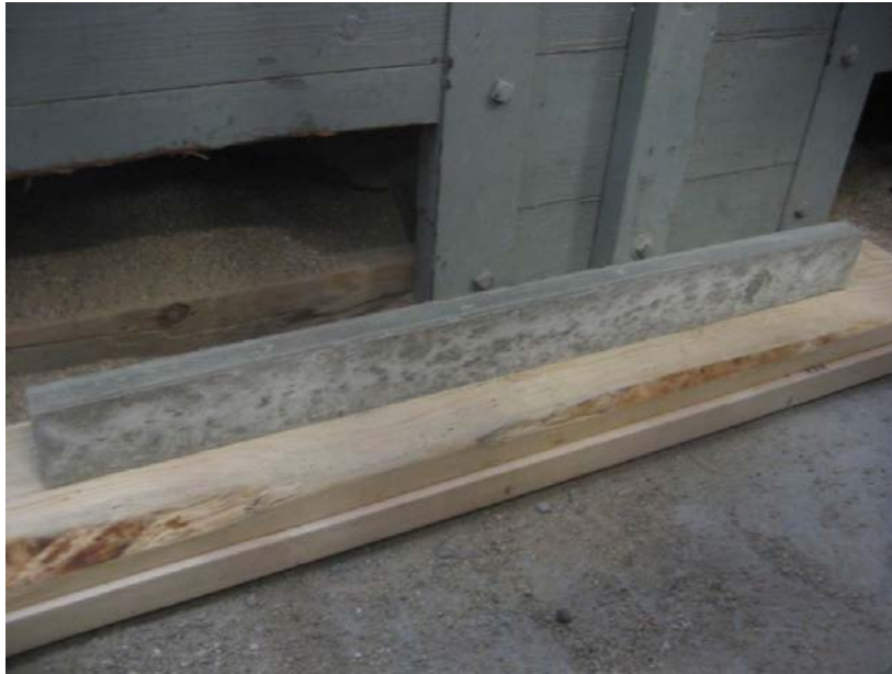
Figure A2. Initial Preliminary Test Setup Mold (The Mold is Upside Down and the Top Side of the Beam when it was in the Mold is now the Largest Face Shown in the Picture)
