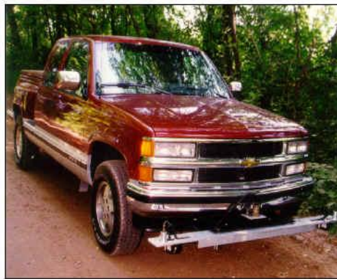
Illustration 2-7. front-mounted laser profiler (Michigan Scientific Corporation, 2005)
