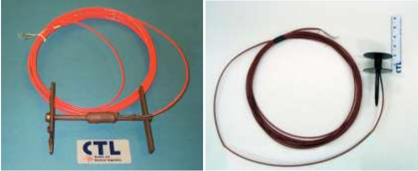
Figure 1: CTL Horizontal and Vertical Strain Gauges
