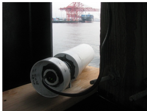
Figure 3.40: Installation of strain gauge (left) and distance sensor (right). Strain gauge covered in silicone and zinc-rich paint to protect against corrosive effects of saltwater. Distance sensor used to record vessel position measurements.
