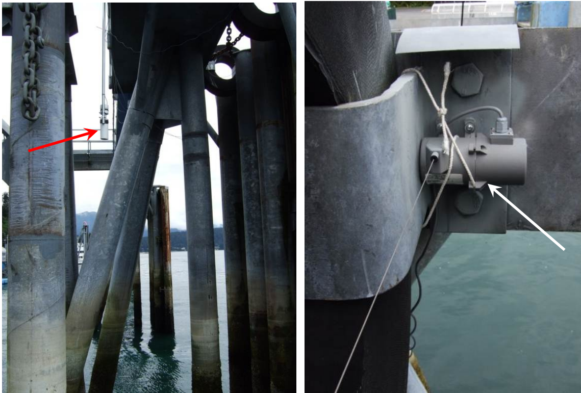
Figure 3.6: Tide gauge (left); LMT (right)
