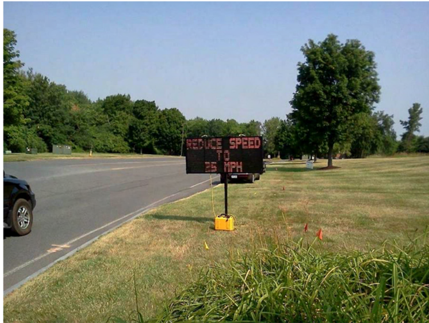
Figure 5-3. Speed display shown in response to speeds greater than 30 mph.
