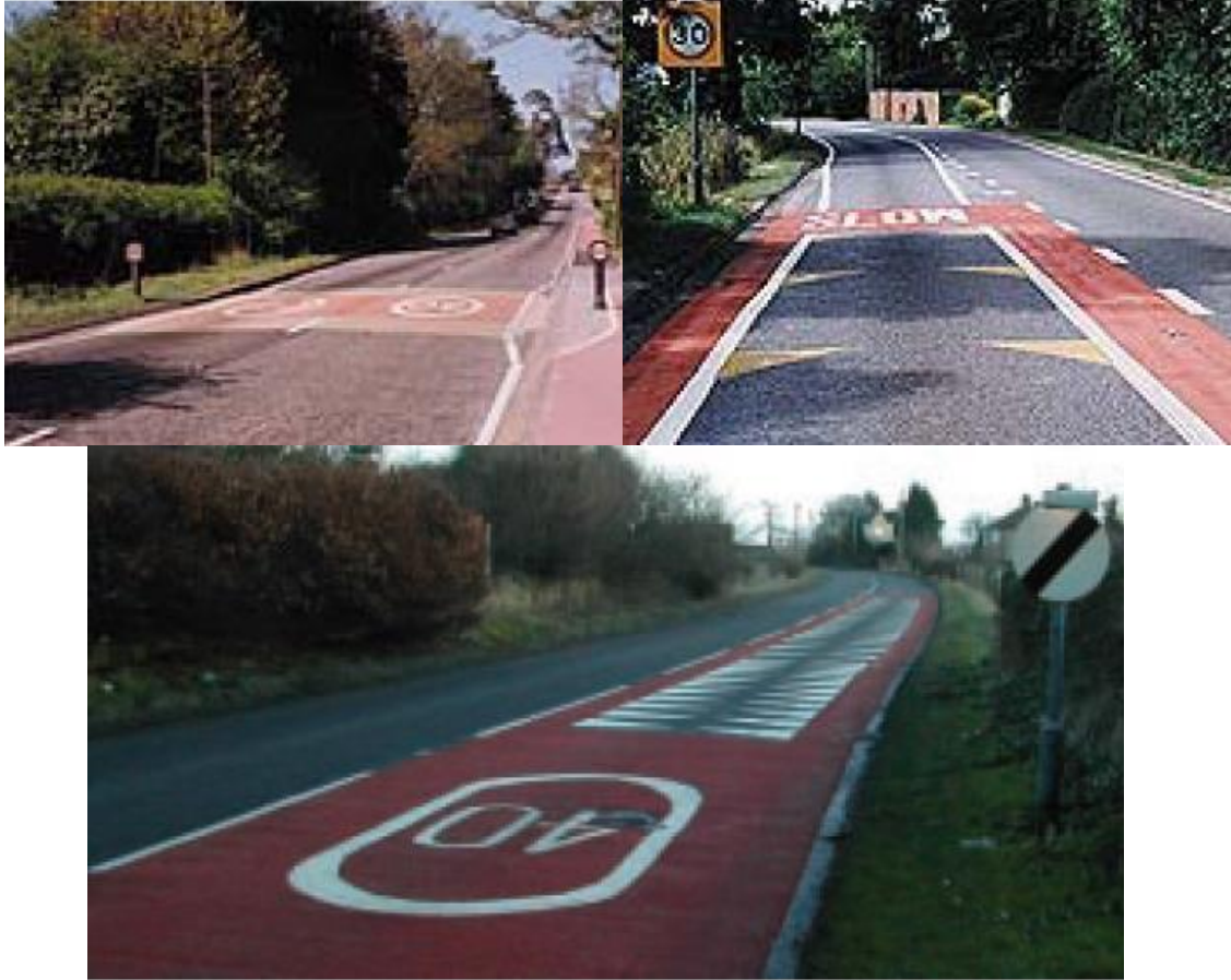
Figure 3-4: Red markings with posted speed limits used in European gateways (Sustrans, 2004)
