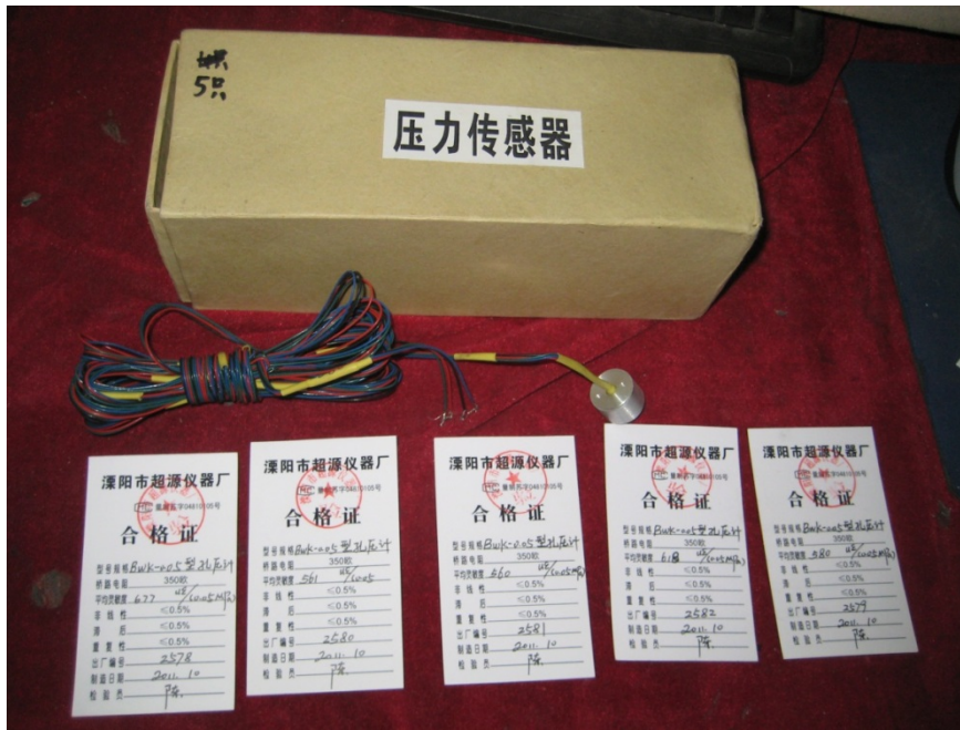
Figure 2.10. Pore pressure sensors
