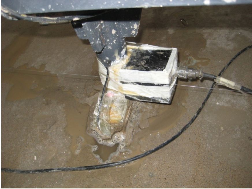
Figure 2.16. Gap formed between the soil and pile, and water spilled out
