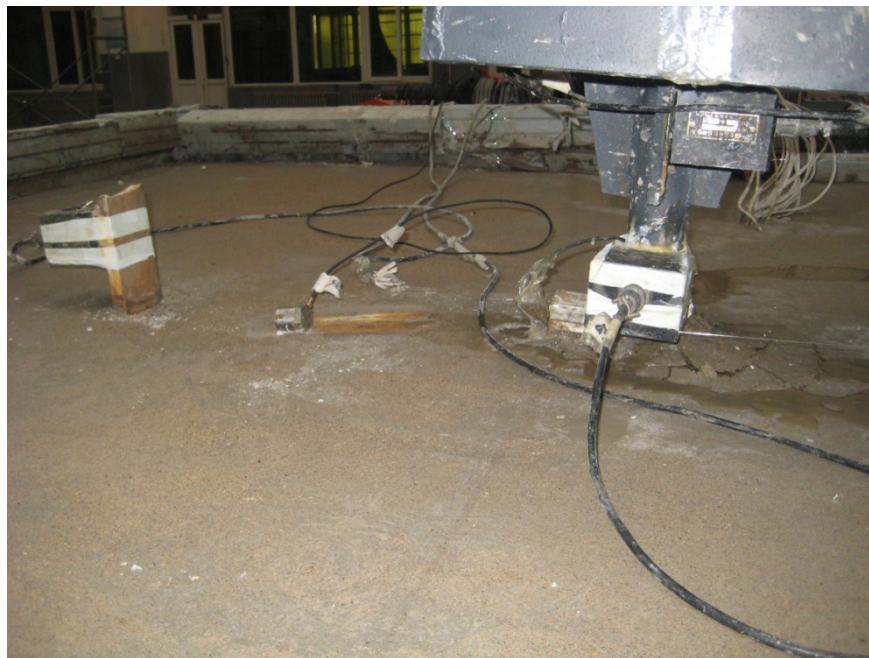
Figure 2.15. Cracks formed near the soil-pile interface
