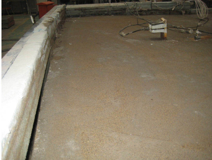
Figure 2.18. Lateral spreading of the simulated frozen crust
