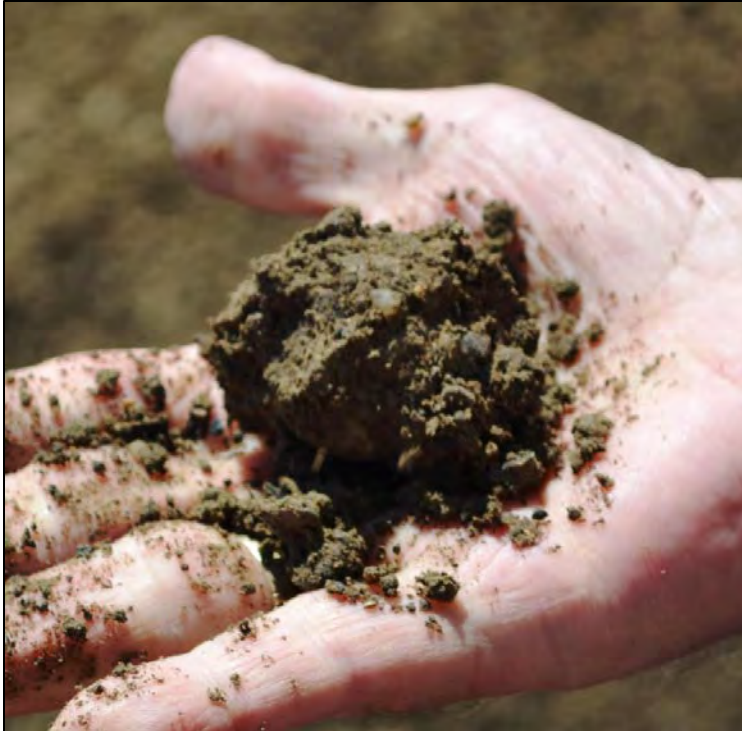
Figure 3.35 Dampened aggregate and RAP blend prepared for application of magnesium chloride and polymer dust suppressant on Sweetwater County's Crooks Gap Road, July 2011.
