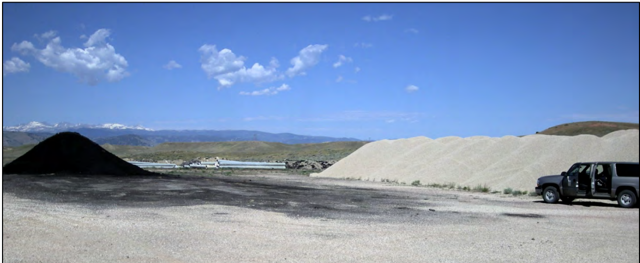
Figure 3.20 RAP and virgin aggregate stockpiles at Johnson County's Piney Creek stockpiles, June 2008.
