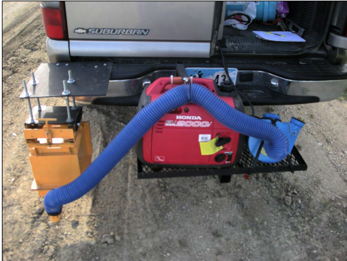
Figure 3.15 Dustometer setup with, left to right, the dustometer, generator, and vacuum.
