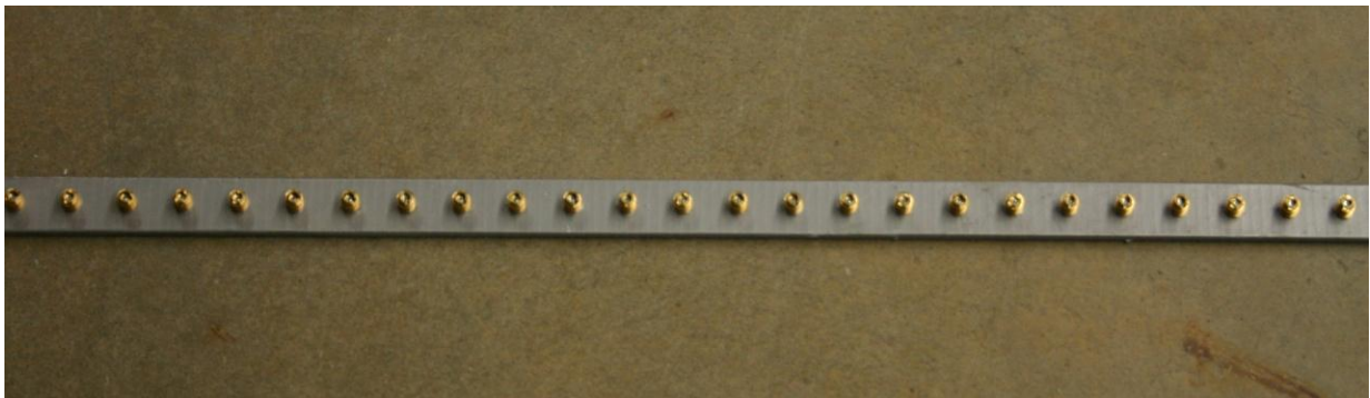
Figure 4.1 Brass points at 1-in. spacing used for Whittemore readings
