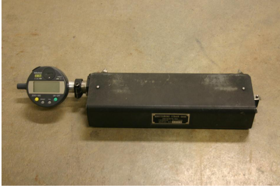
Figure 4.3 Whittemore gage used to take readings
