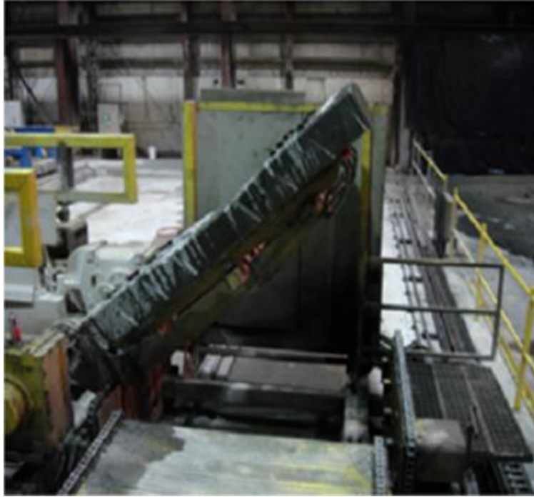
Figure 3.9 Vacuum lifting of ties
