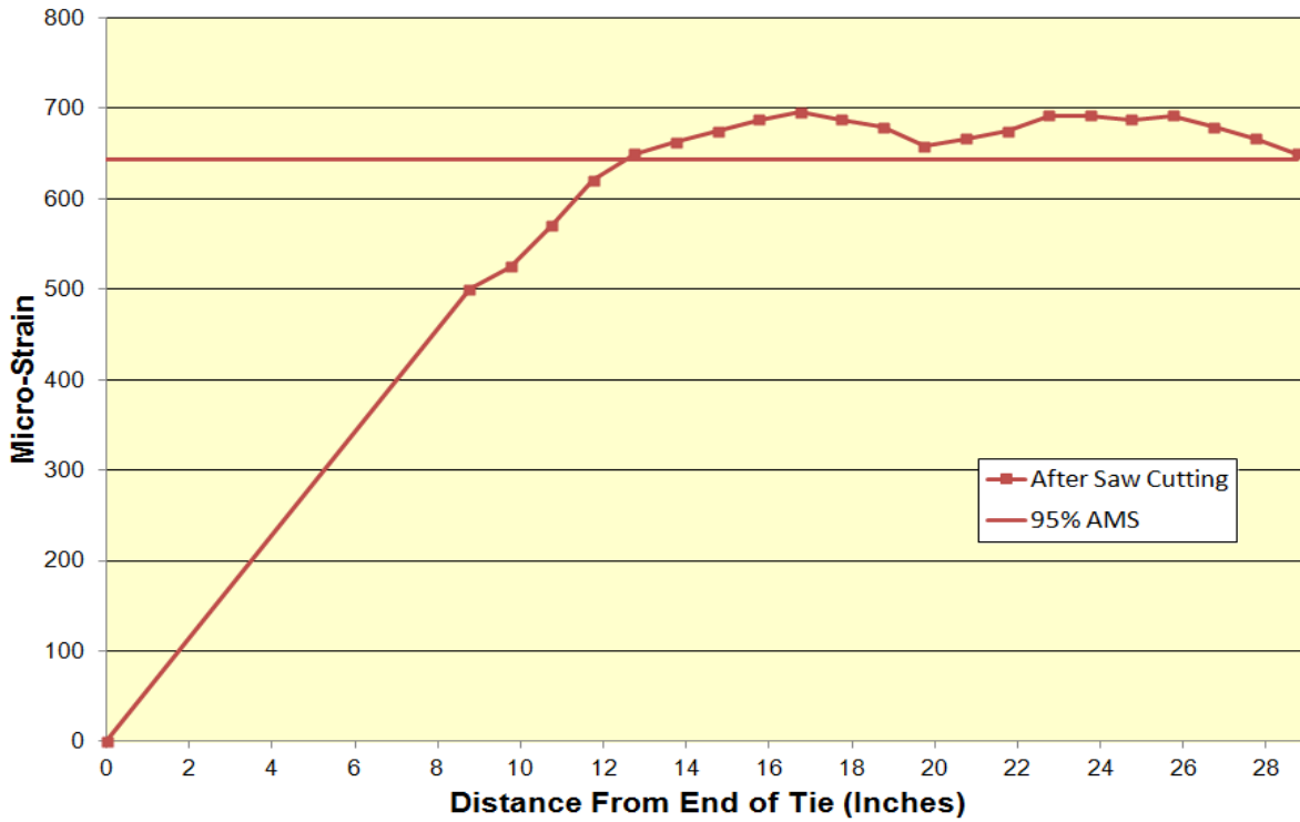
Figure B.29 Transfer length of Plant B Mix 3/RF 3 Tie 23A
