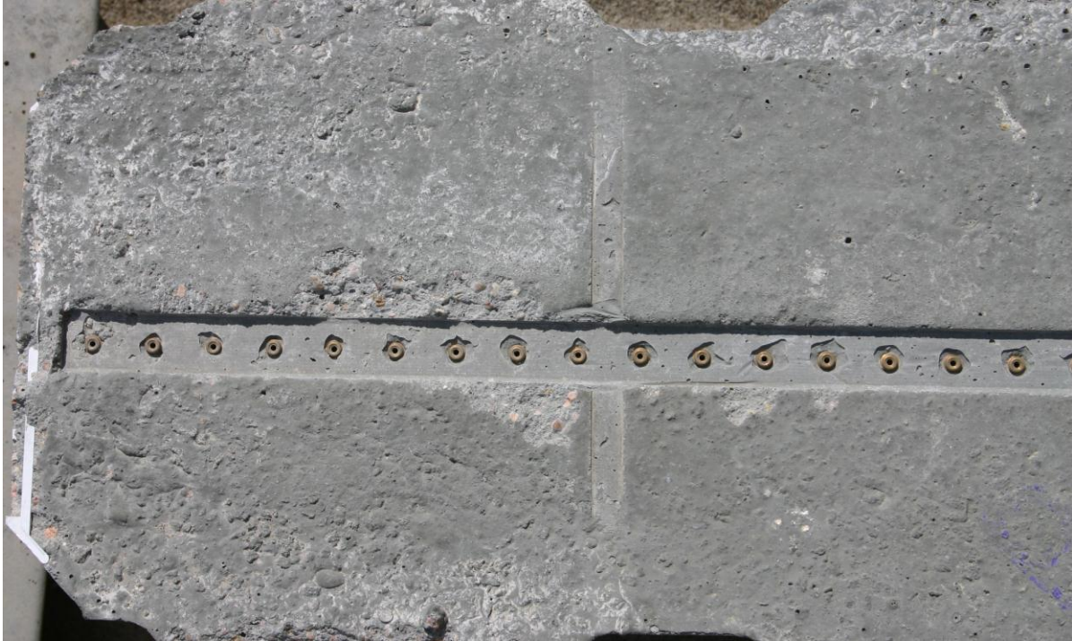
Figure 4.2 Embedded brass points used for Whittemore readings
