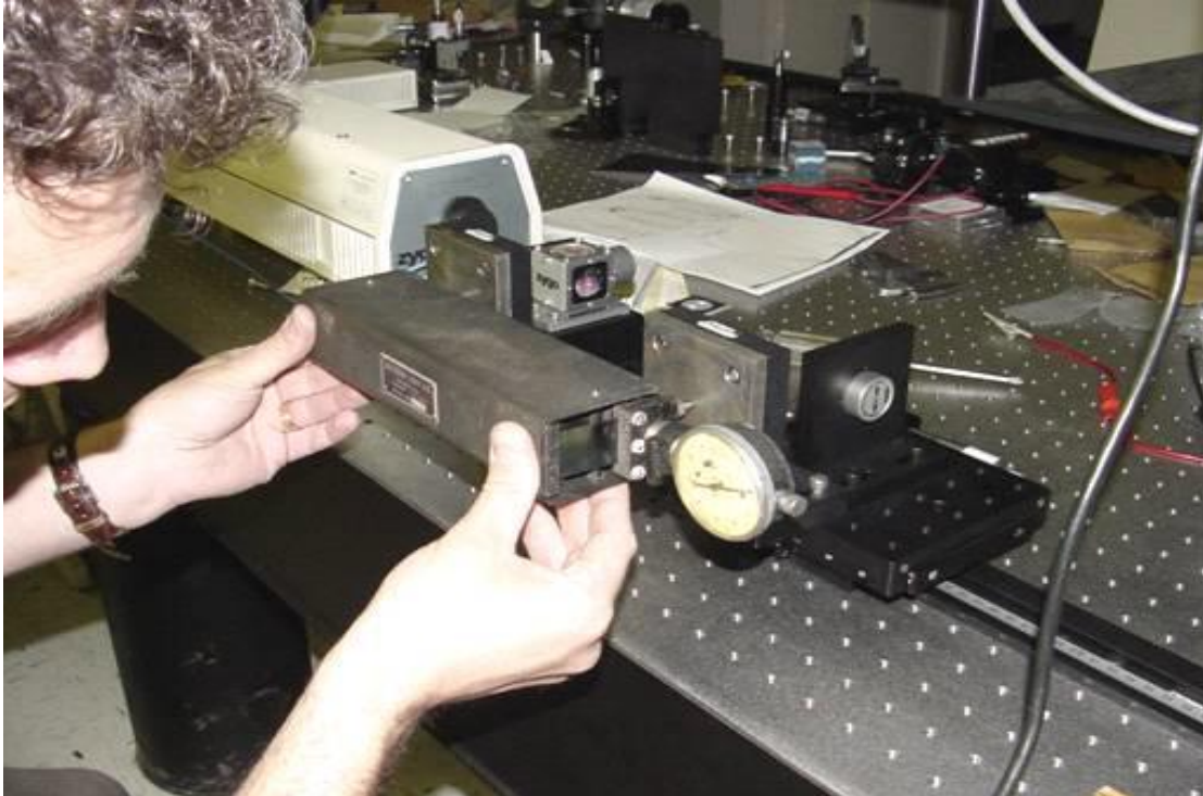
Figure 3.3 Determining accuracy of a standard mechanical gage (Zhao 2011)
