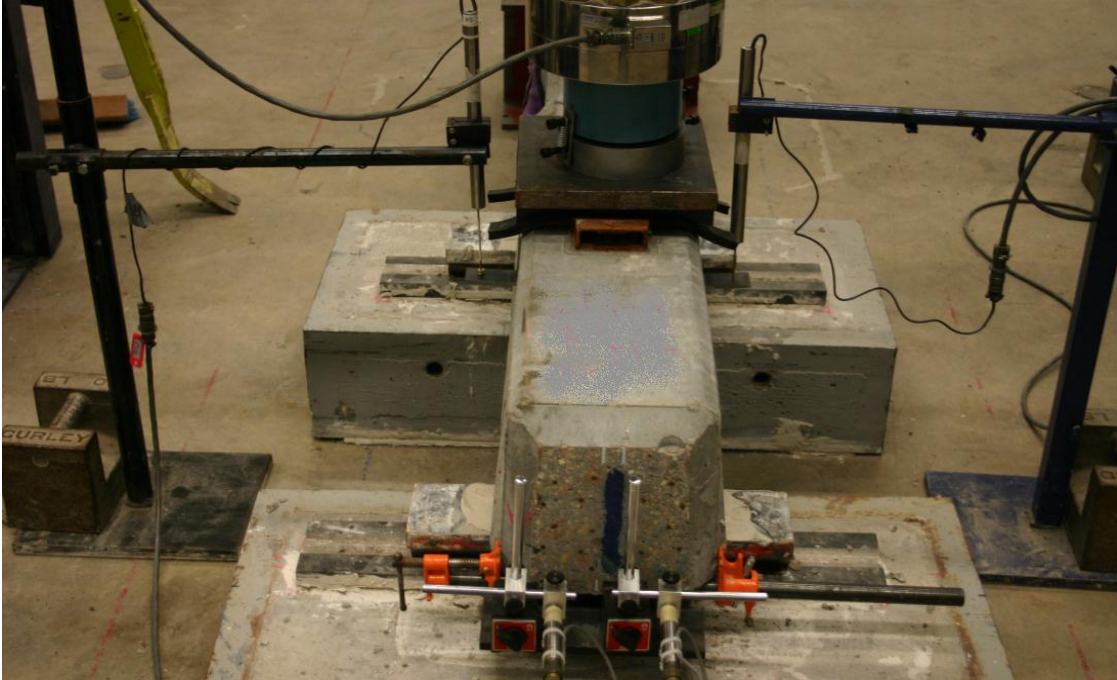
Figure 7.5 Setup of rail seat positive moment test
