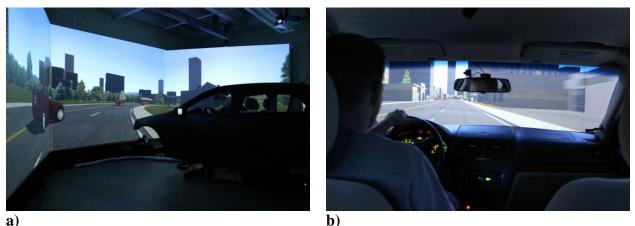
*Figure 1:* Example a) layout of the Realtime Technologies Inc. driving simulator utilizing the SimVista driving simulator software and a view b) from inside the simulator.
