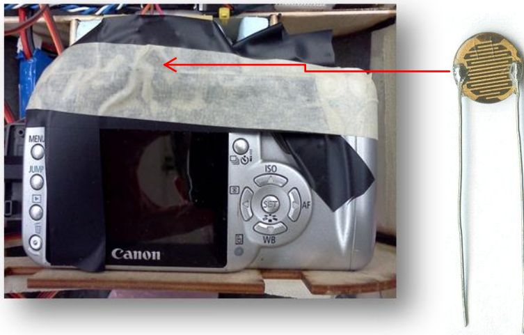
Fig. 10. Photoresistor Installed in a Digital SLR Rangefinder
