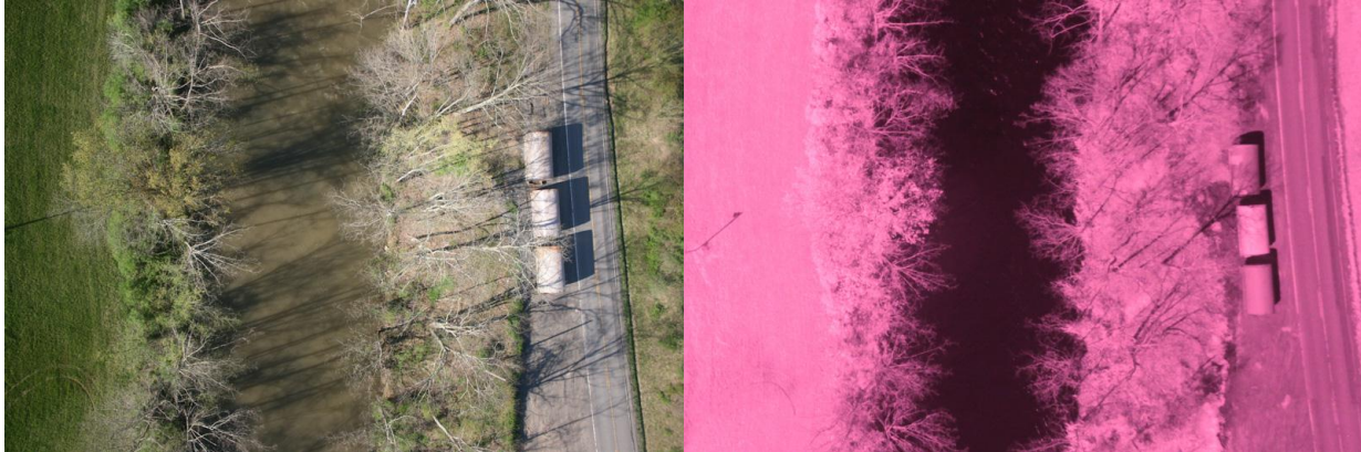
Fig. 16. Aerial Photos of the Same Region with Visible Spectrum and Near-IR
