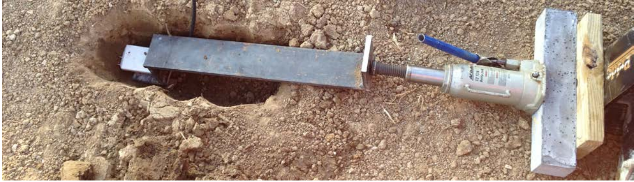
Figure 3.16. Installation of TDR probe in Pad 1.
