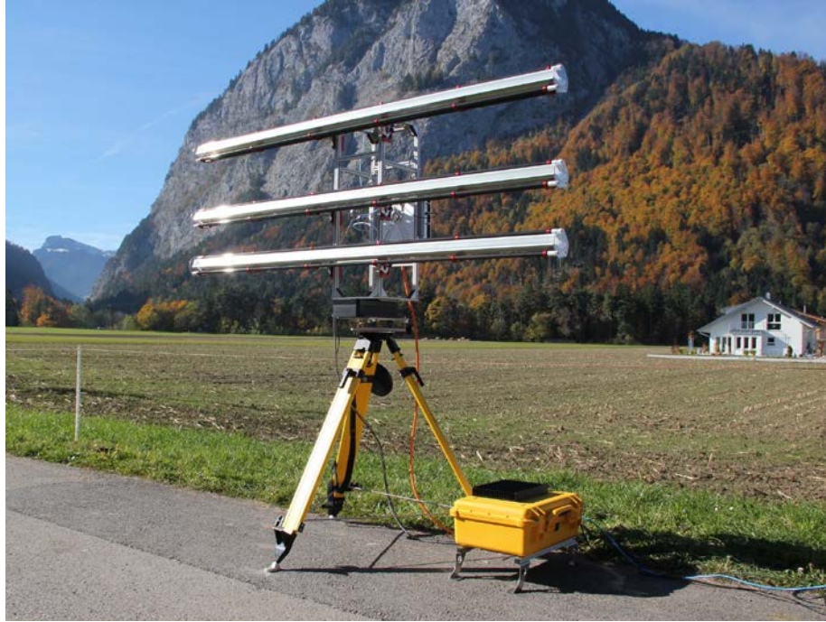
Figure 2.9. GPRI-II acquiring images of a mountain near Gumligen, Switzerland on October 31, 2010 (from GAMMA Remote Sensing AG, 2011 as cited by Conte, 2012).
