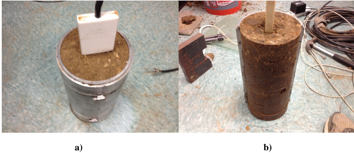
Figure 4.2. a) Prepared sample in split mold. b) Prepared sample with mold partially removed.
