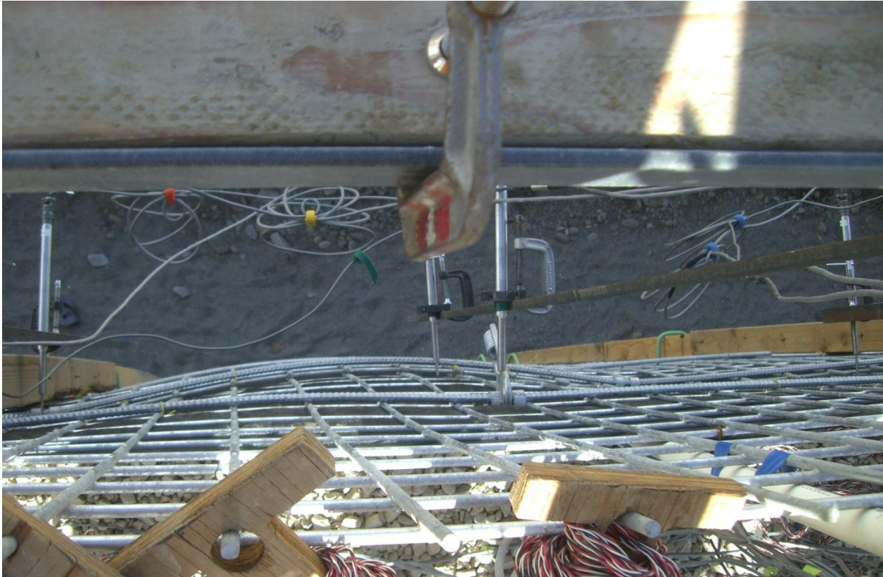
Figure 5.48: View from above of the wall displacement and LVDTs for pile TP8
