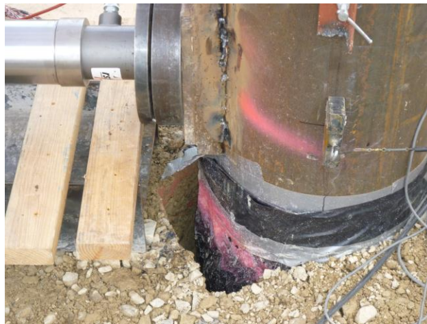
Figure 3.11: Double LDPE sheeting wrapped around TP3.
