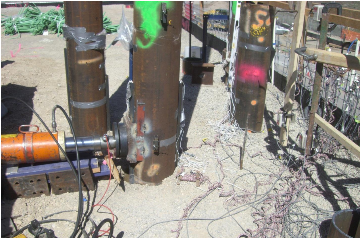
Figure 5.40: A view of the displacement of pile TP8 during loading
