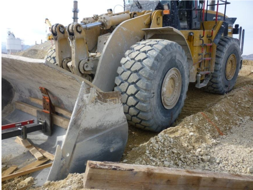
Figure 5.4: Reaction for load at TP4 up to 0.75 in. displacement (Pioneer Crossing Site).
