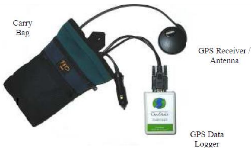
Figure 4-4. In-vehicle GeoLogger (source: GeoStats)
