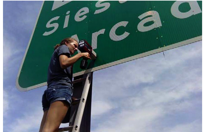
A technician measures the retroreflectivity of a sign in southwest Florida.
