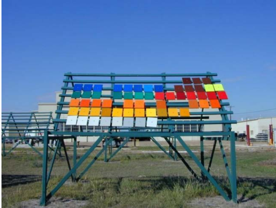
Figure 3.4 Weathering Racks Used for Accelerated Sign Degradation
