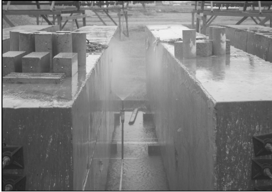
Figure 2-5. Sprinkler System between Two Specimens Load Testing Results.
