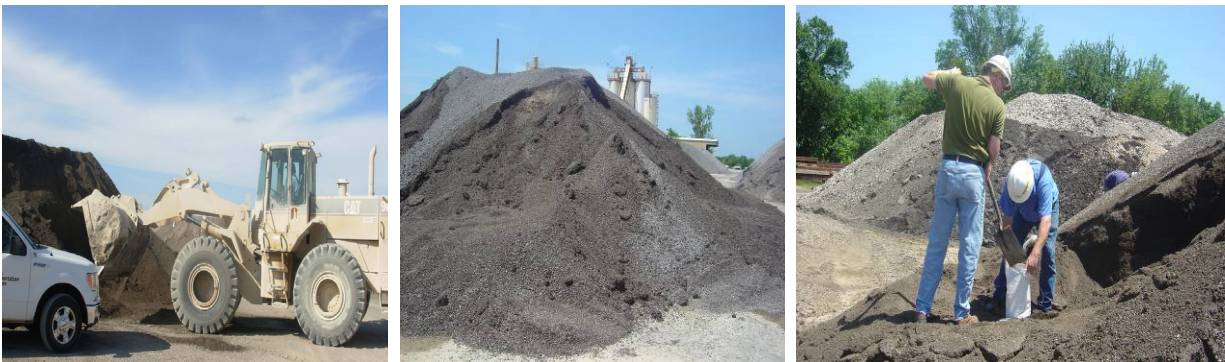
Figure A1. Sampling RAP Stockpiles.
