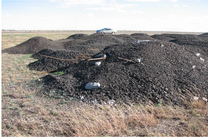
Figure A1. Contaminated RAP Stockpile.
