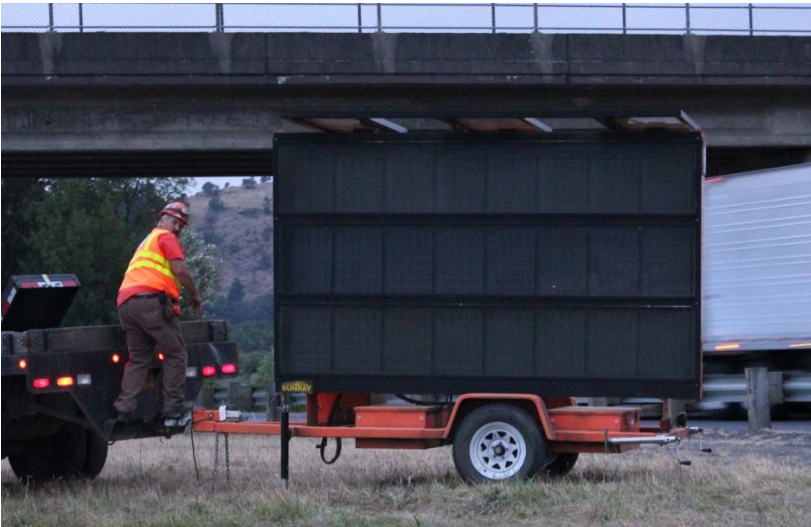
Figure 2.9: PCMS on Trailer
