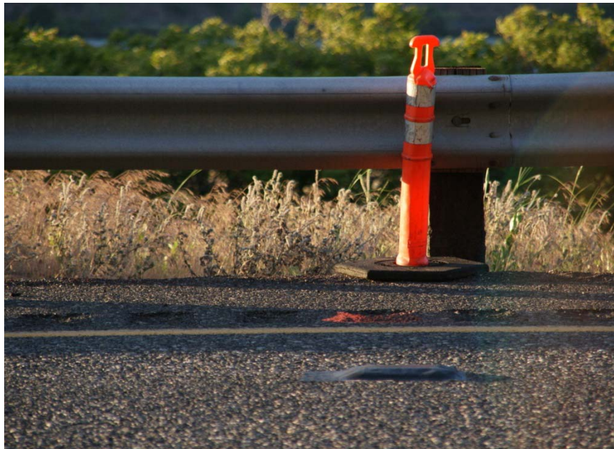
Figure 3.6: Placement of Portable Traffic Analyzer by Adhesive Tapes
