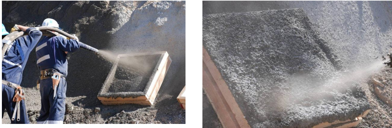
Figure 10. Casting of Shotcrete FRC Samples for Flexural and Compressive Strength Testing.
