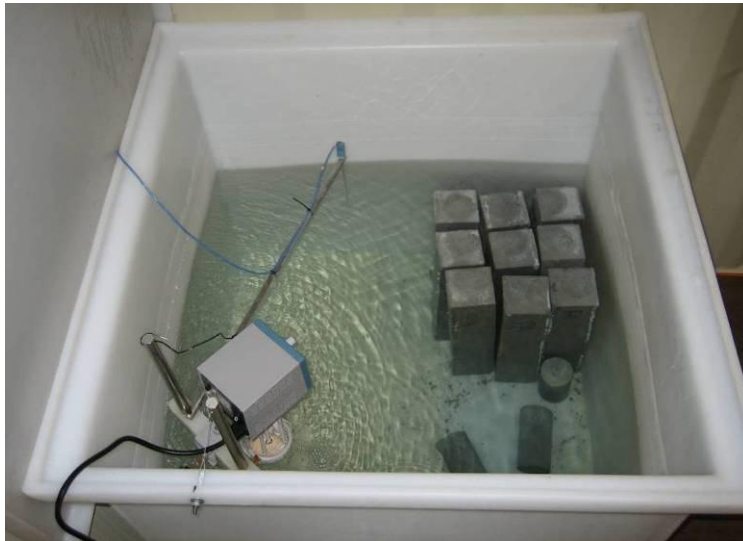
Figure 34. Curing of Specimens in the Water Tank at a Constant Temperature of 70° F.
