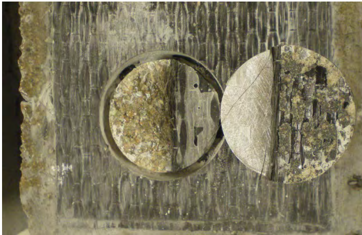
Figure 6.28 Combined Mode A and Mode F Failure
