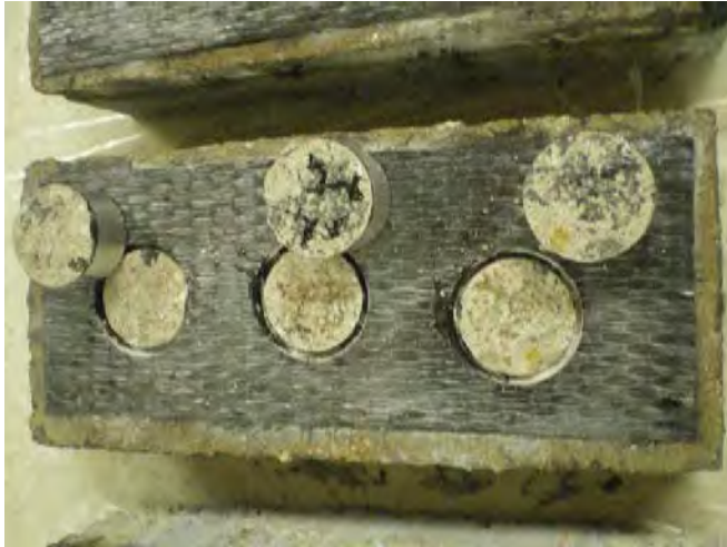
Figure 6.25 Mode F failures (ASTM D7522) during Stage 1 testing
