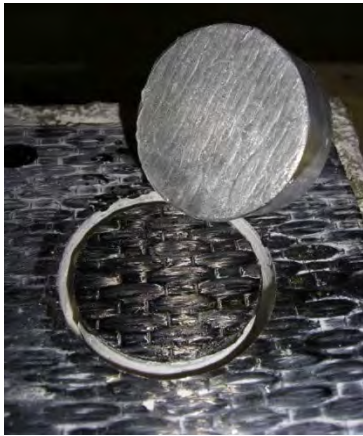
Figure 6.18 Pull-off Mode A failure
