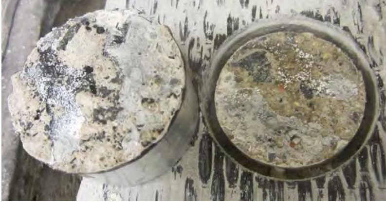
Figure 6.32 Presence of moisture on Dollies
