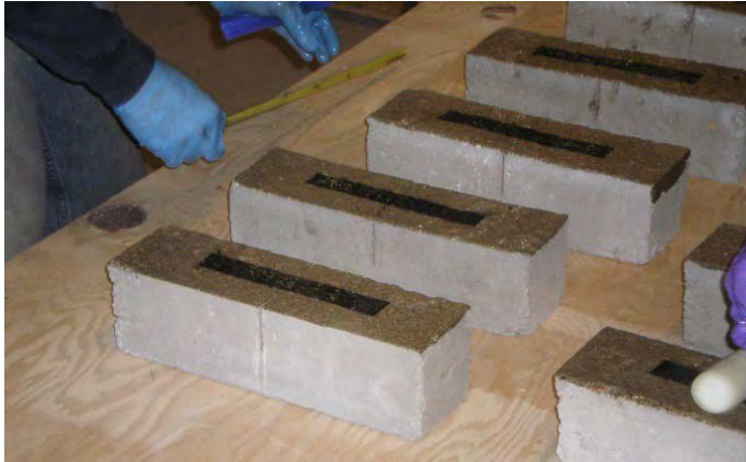
Figure 6.15 Concrete beams reinforced with CFRP
