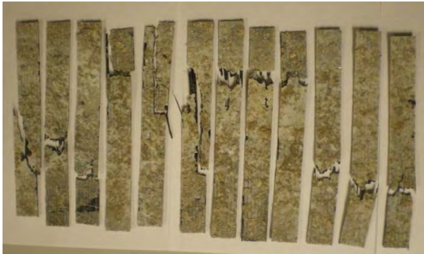
Figure 4.2 Failed tensile test specimens from the large void removed from bay 3NE. Note the oatmeal appearance
