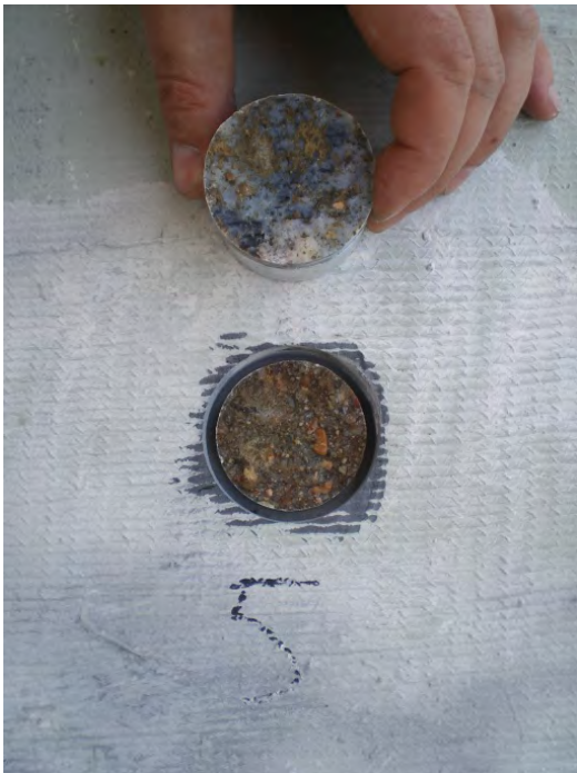
Figures B12 and B13. Test No.14, weak bond strength, and Test No.15, weak bond strength Test No.16 Not available, puck had faulty threads
