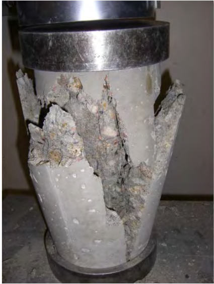
Figure 6.17 Characteristic failure for compression tests
