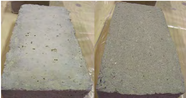
Figure 6.10 Concrete surface before (left) and after (right) sandblasting
