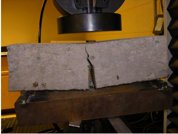
Figure 6.22 Beam following crack failure
