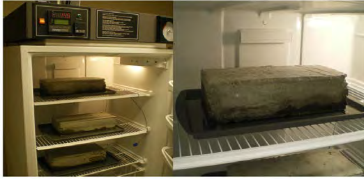
Figure 6.7 FRP Reinforced concrete specimens undergoing free-thaw exposure
