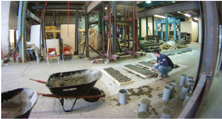
Figure 6.8 Casting of concrete specimens
