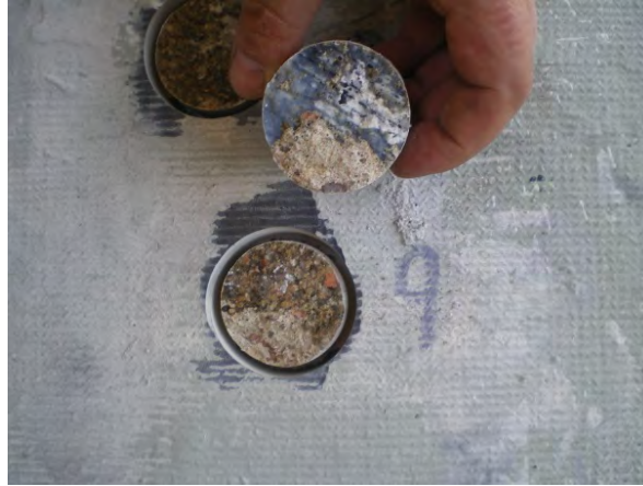
Figure B8. Test No.9, weak bond strength
