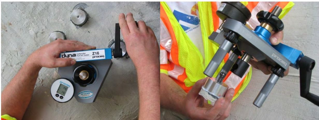
Figure 3.13 Conducting a pull-off test with the digital manometer reading and removing the tested puck from the pull-off tester
