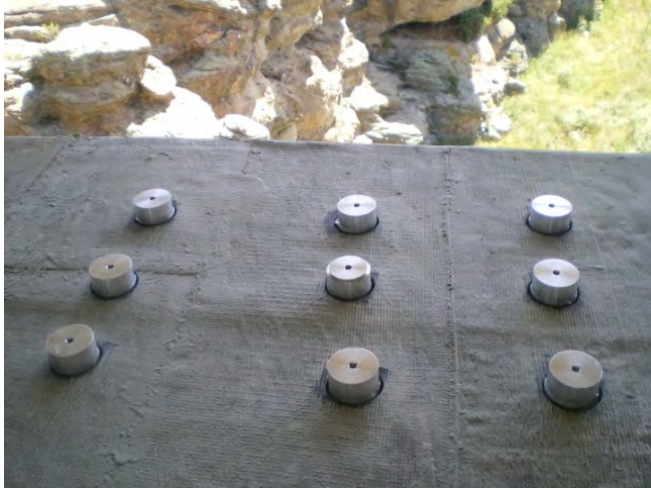
Figure 3.11 Adhered aluminum pucks for pull-off tests
