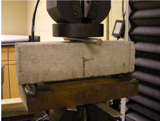
Figure 6.16 Beam fixture and specimen
