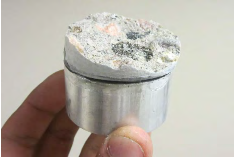
Figure 6.31 Mode G Failure in Dolly #20
