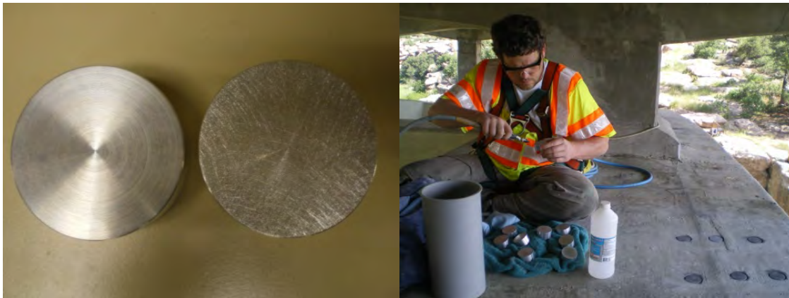
Figure 3.10 Aluminum pucks before and after sanding with 40 grit sandpaper and preparing the aluminum pucks way up high on the arch
