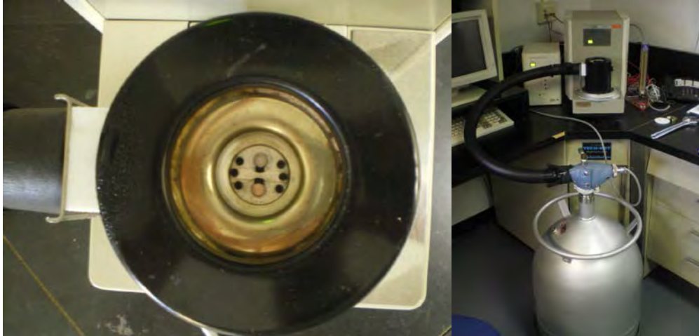
Figure 4.12 DSC specimen chamber and DSC with liquid nitrogen
