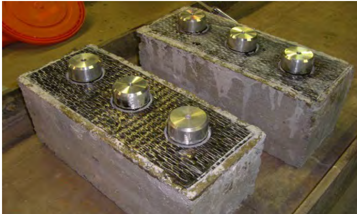
Figure 6.13 Concrete specimens following adhesion of dollies
