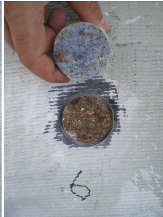
Figures B12 and B13. Test No.14, weak bond strength, and Test No.15, weak bond strength Test No.16 Not available, puck had faulty threads
