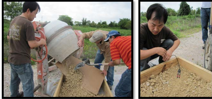
Figure 3.1. Placing Test Box Material in Lifts and Inserting FDR Probes.
