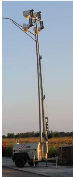
Figure 16. Trailer-Mounted Light Tower.
