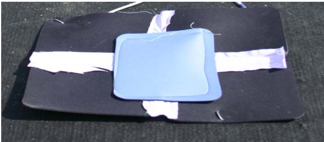
Figure 3.14. Geotextile strain gage protection, neoprene pad (Howard 2006).
