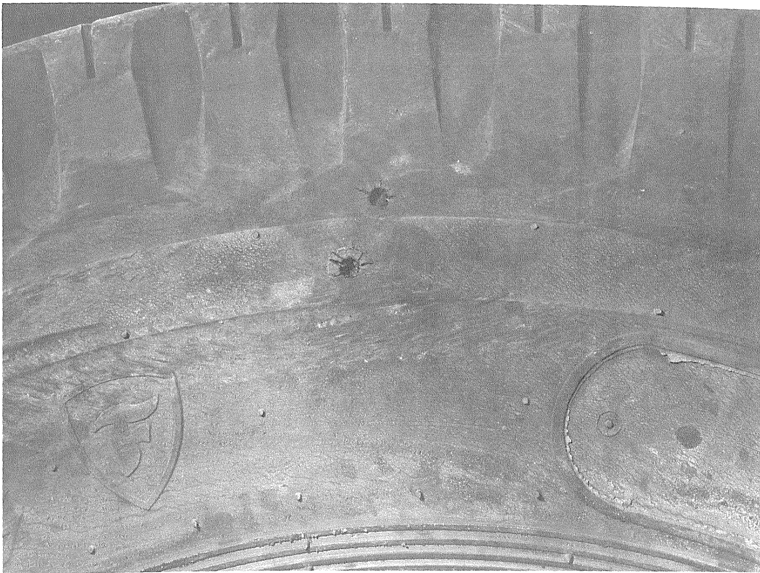
Figure 5-5. Typical Post-test Point of Entry Holes for Deflation Projectiles.
