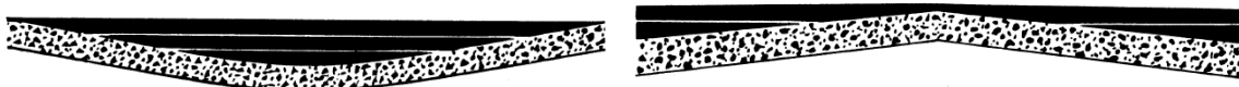
Figure 2-2. Illustration of the Correct Way to Place Level-up Patches in Sag or Excessive Crown Areas (after Asphalt Institute 1974).
