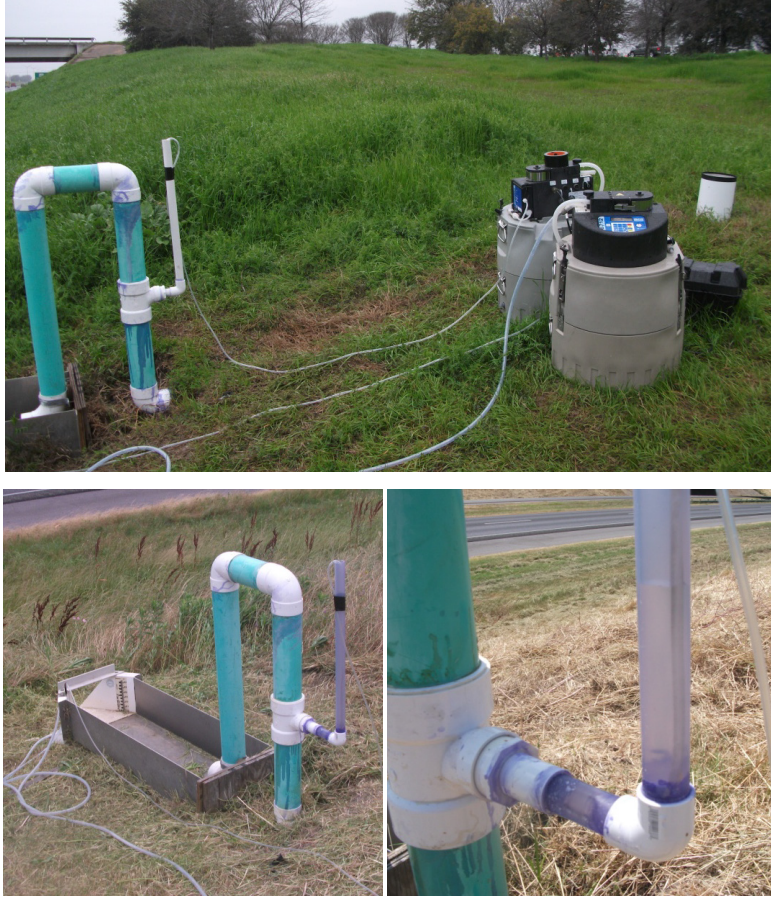
Figure 11. Modification of Effluent Discharge to Create IWS Layer.
