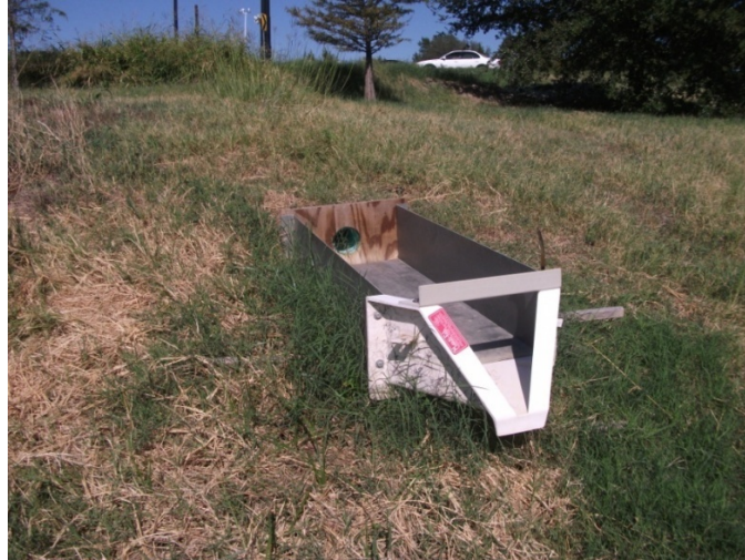
Figure 10. H-Flume Installed at the Effluent Location to Measure Flow.
