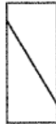
Type 4 Diagonal fracture with no cracking through ends; tap with hammer to distinguish from Type 1
