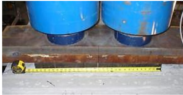
Figure 30–Support conditions at load point for specimen LB
