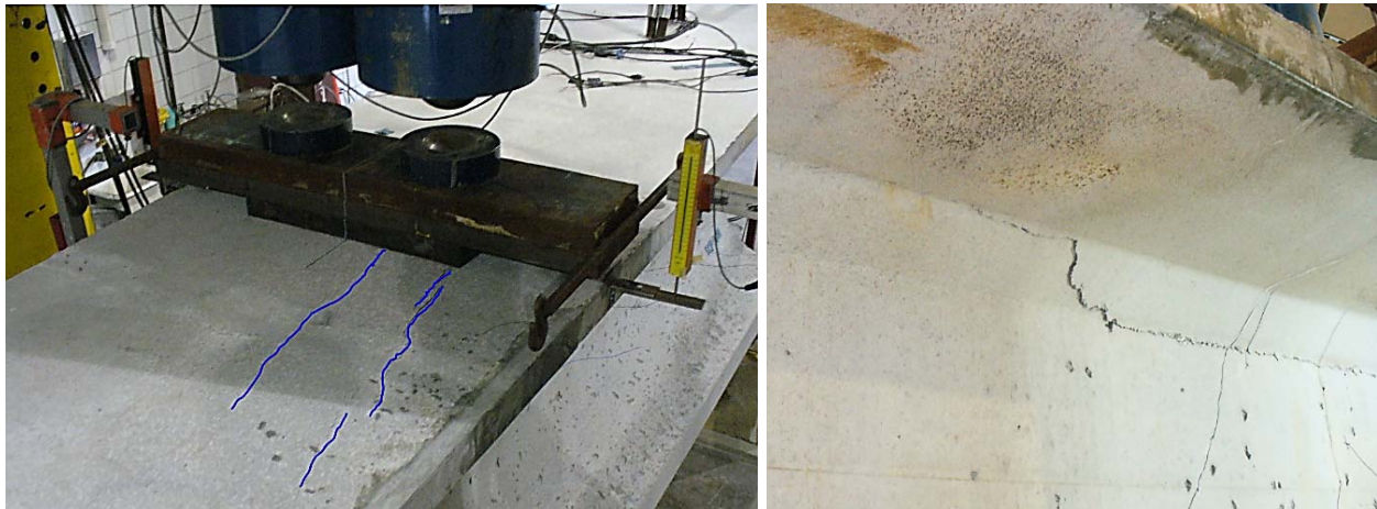
Figure 77–Punching failure from above (left) and below (right)
