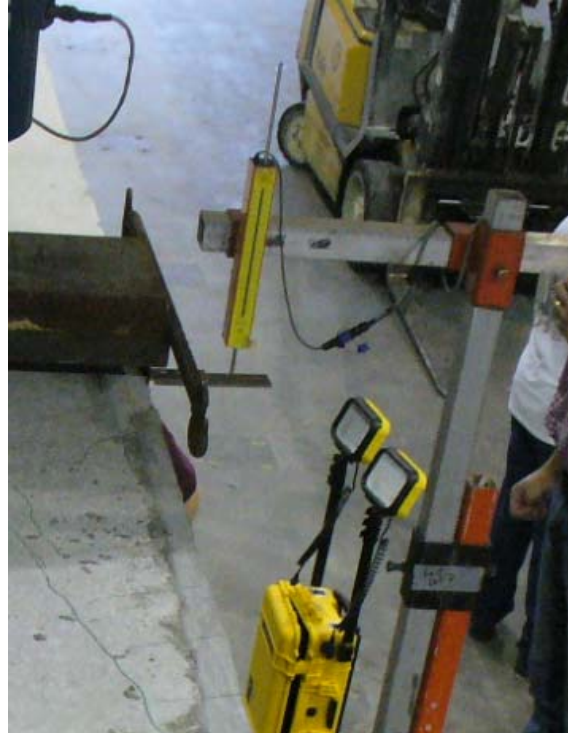
Figure 40–LVDT and support frame
