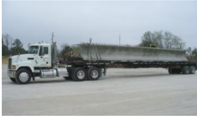
Figure 31–Girder H on truck prior to transit
