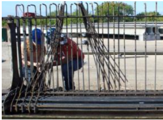
Figure 21–Girder W reinforcement A) Specimen WN and B) Specimen WB
