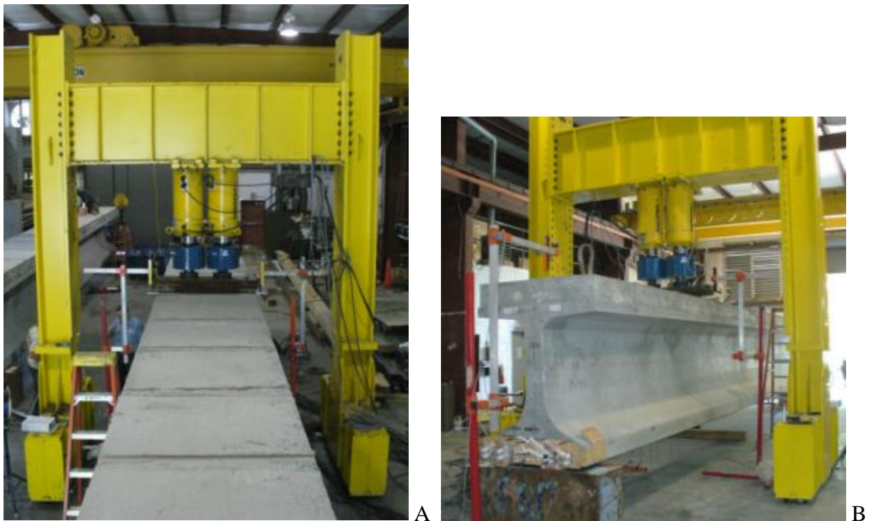
Figure 36–Test specimen and load frame A) top of girder and B) end of girder.
