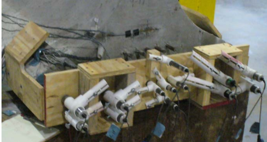
Figure 47–Wood frame and LVDTs
