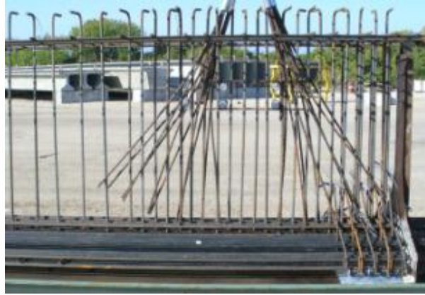
Figure 21–Girder W reinforcement A) Specimen WN and B) Specimen WB
