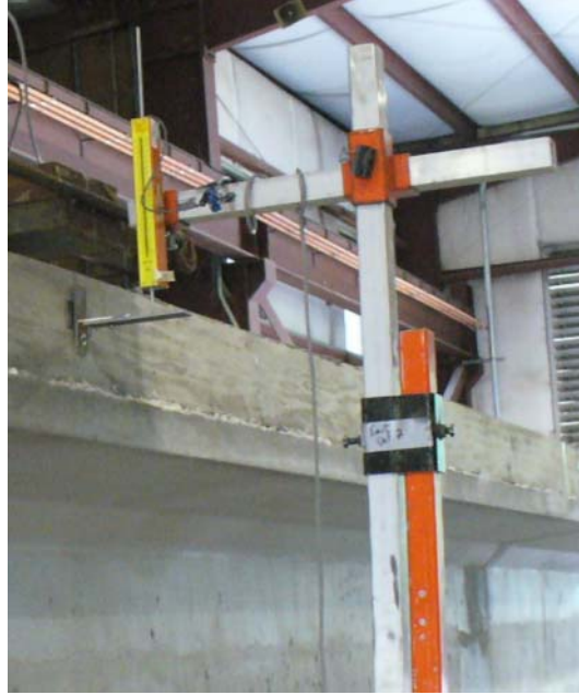
Figure 45–LVDT and support frame
