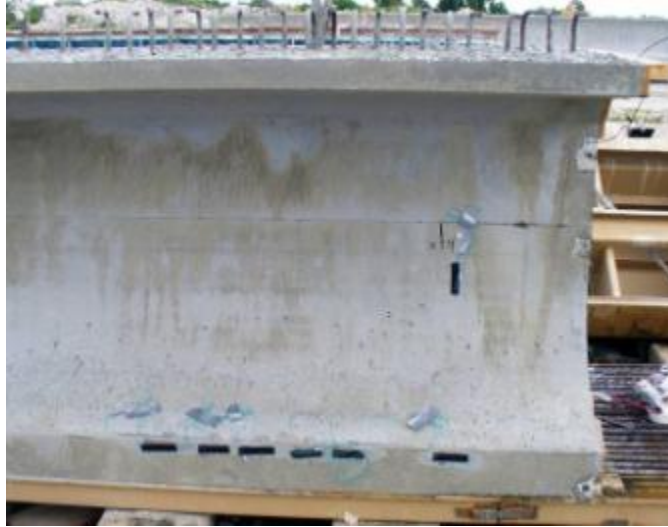
Figure 66–Strain gages for measuring transfer length
