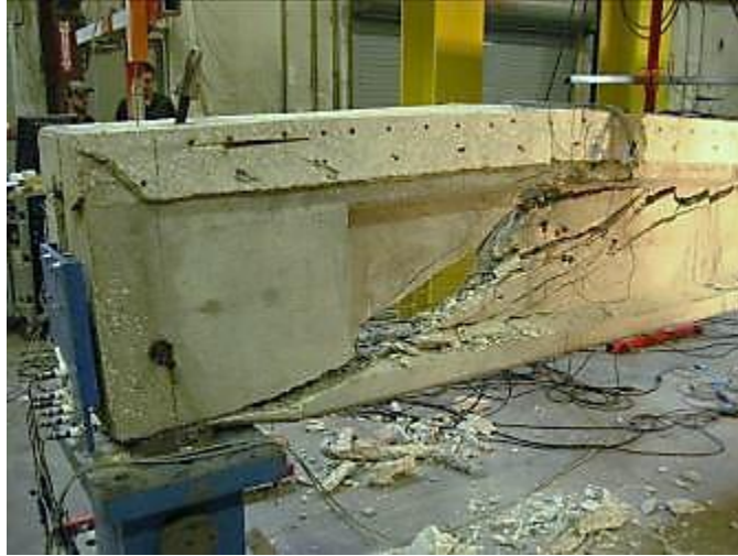
Figure 29-I2A incline cracks in web
