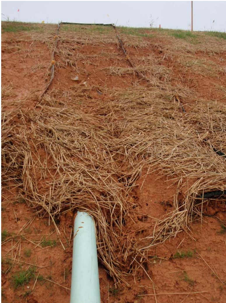
Figure A11: Example of plot failure at planned site 2 (Asheboro, N.C.). The site was abandoned after this first event.
