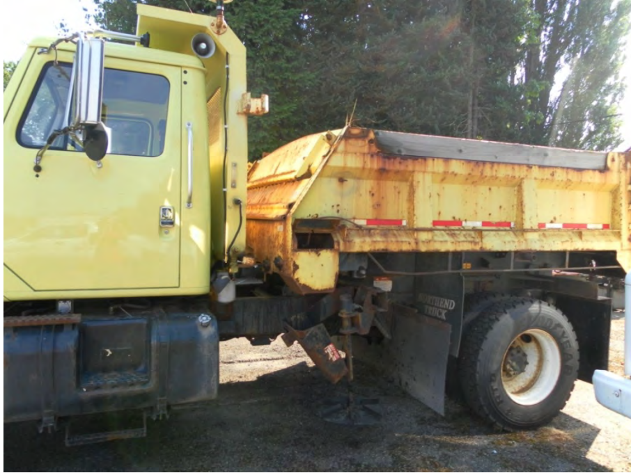
Figure 36. Side discharge salt spreader showing extensive corrosion.
