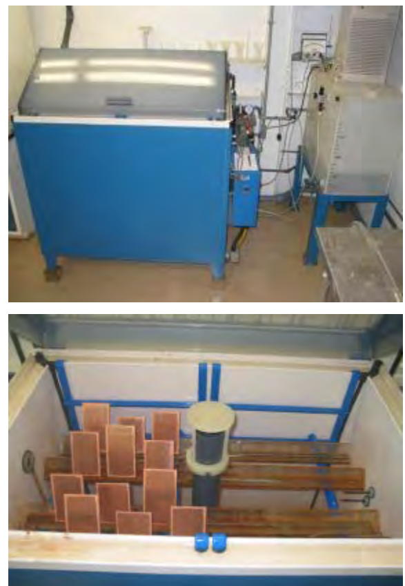
Figure 3. ASTM B117 test chamber and various specimens as loaded into the salt spray.
