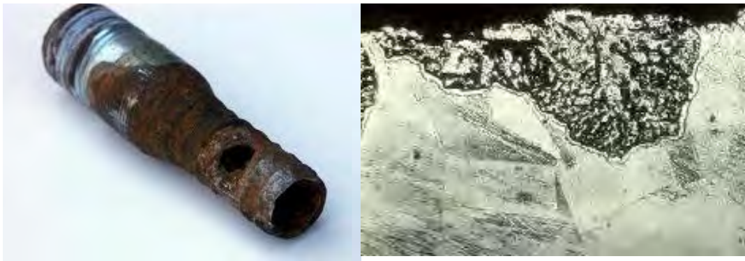
Figure 6 Erosion corrosion (Kopeliovich, 2009)
