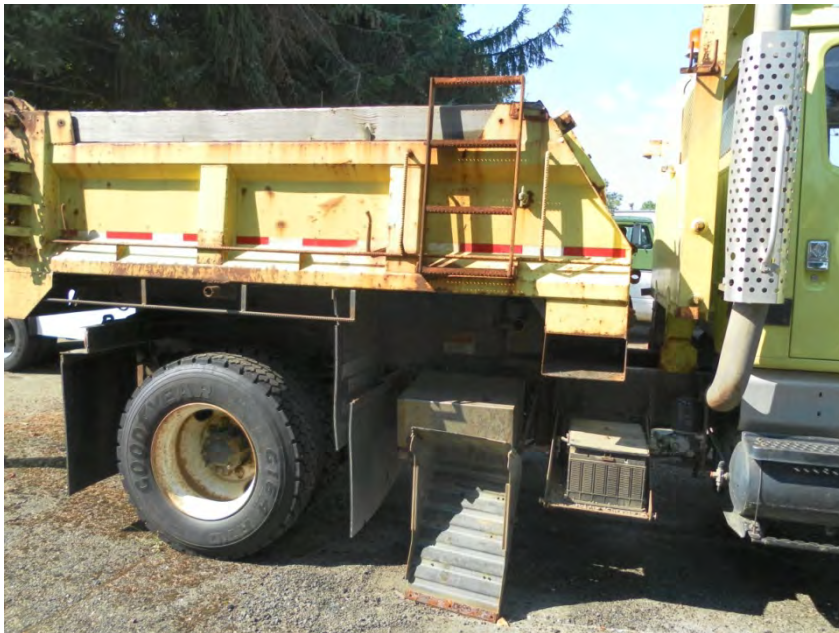
Figure 39. Protective cover for battery.
