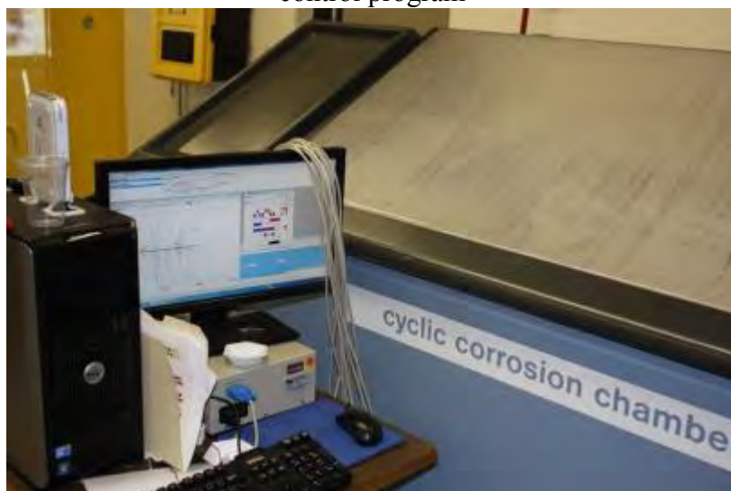
Figure 6. Photographic illustration of the cyclic corrosion chamber (Humid Stage) and MMA data acquisition system
