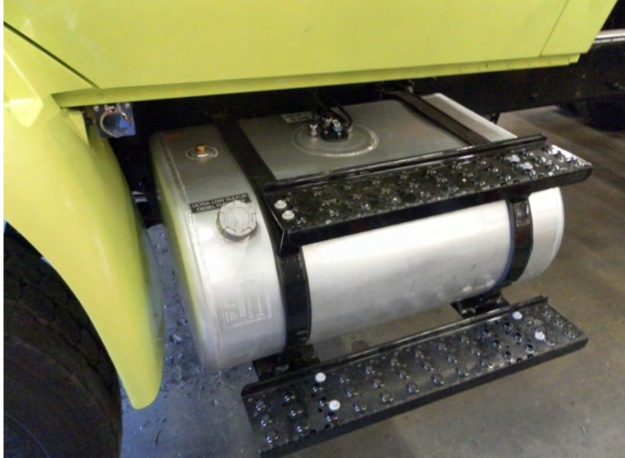
Figure 42. New aluminum fuel tanks.
