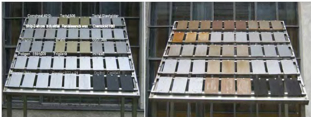
Figure 3: Three panels of each coating were subjected to atmospheric corrosion testing. The panels were mounted on two frames in June 2009 (left). The same panels show discoloration and the formation of corrosion by December 2009 (right) [71].
