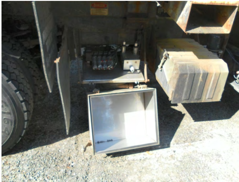
Figure 37. Hydraulic components protected from corrosion using modified sealed protective cover.
