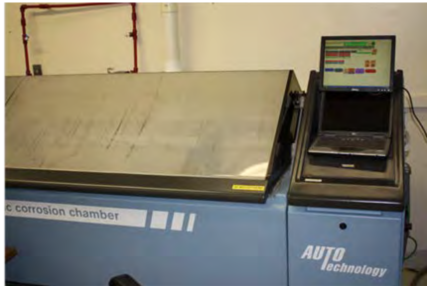
Figure 5. Photographic illustration of the cyclic corrosion chamber (Humid Stage) and control program
