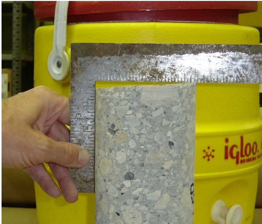
Figure 6 Skew on bottom of core.
